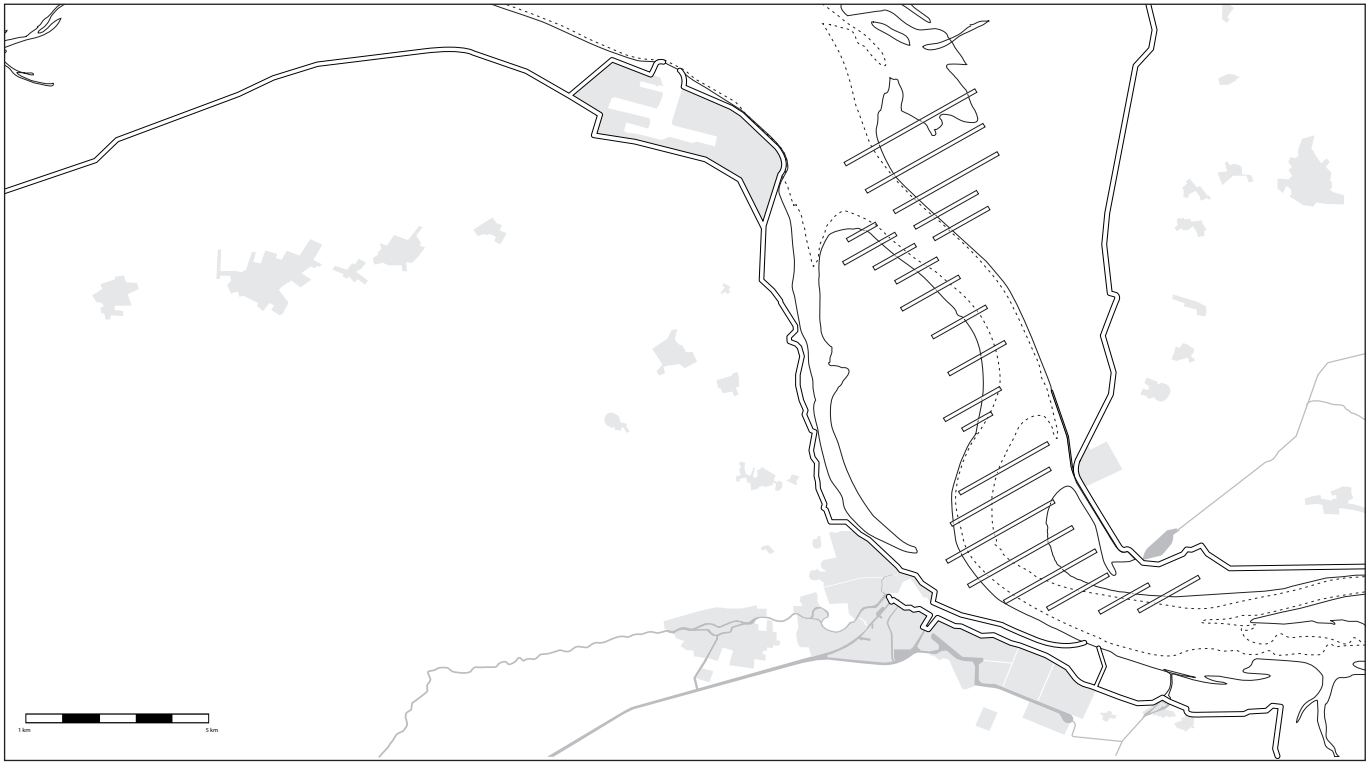
Figure 5.14(above) and 5.15(down) | Fase III. Extending the groynes ensures: an even more intense meander, further narrowing of the shipping channel and a broader side channel.
