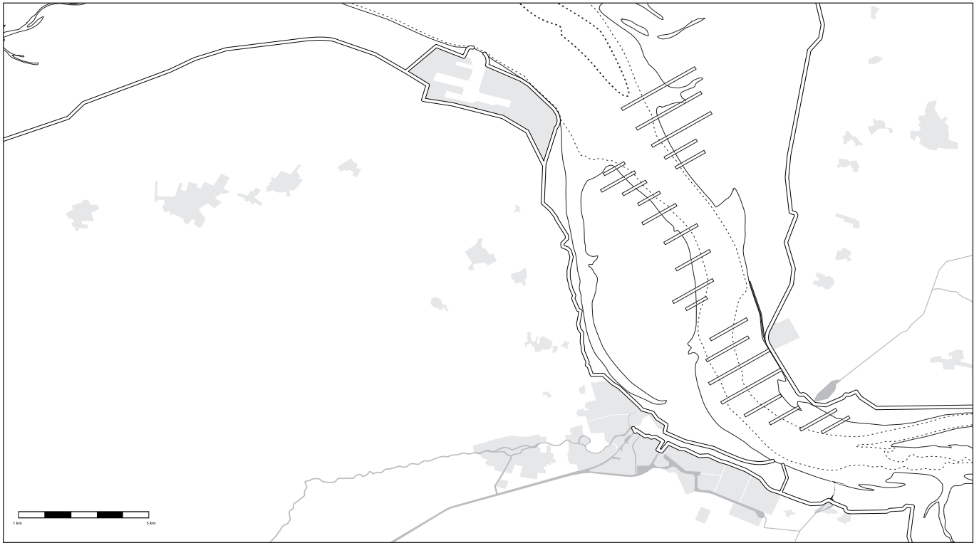
Figure 6.12(above) and 6.13(down) | Fase II. Extending the groynes ensures: a more intense meander, narrowing of the shipping channel and a broader side channel.
