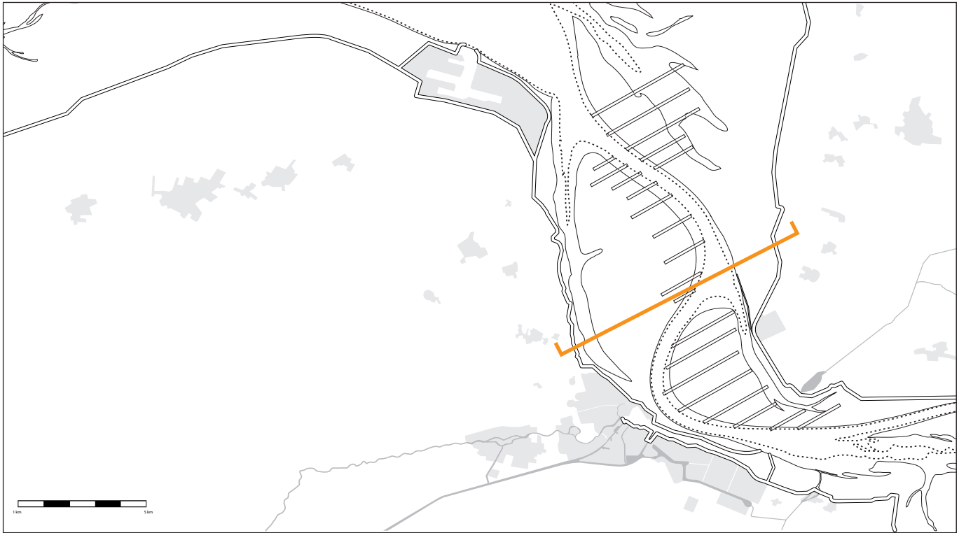
Figure 5.14(above) and 5.15(down) | Fase III. Extending the groynes ensures: an even more intense meander, further narrowing of the shipping channel and a broader side channel.
