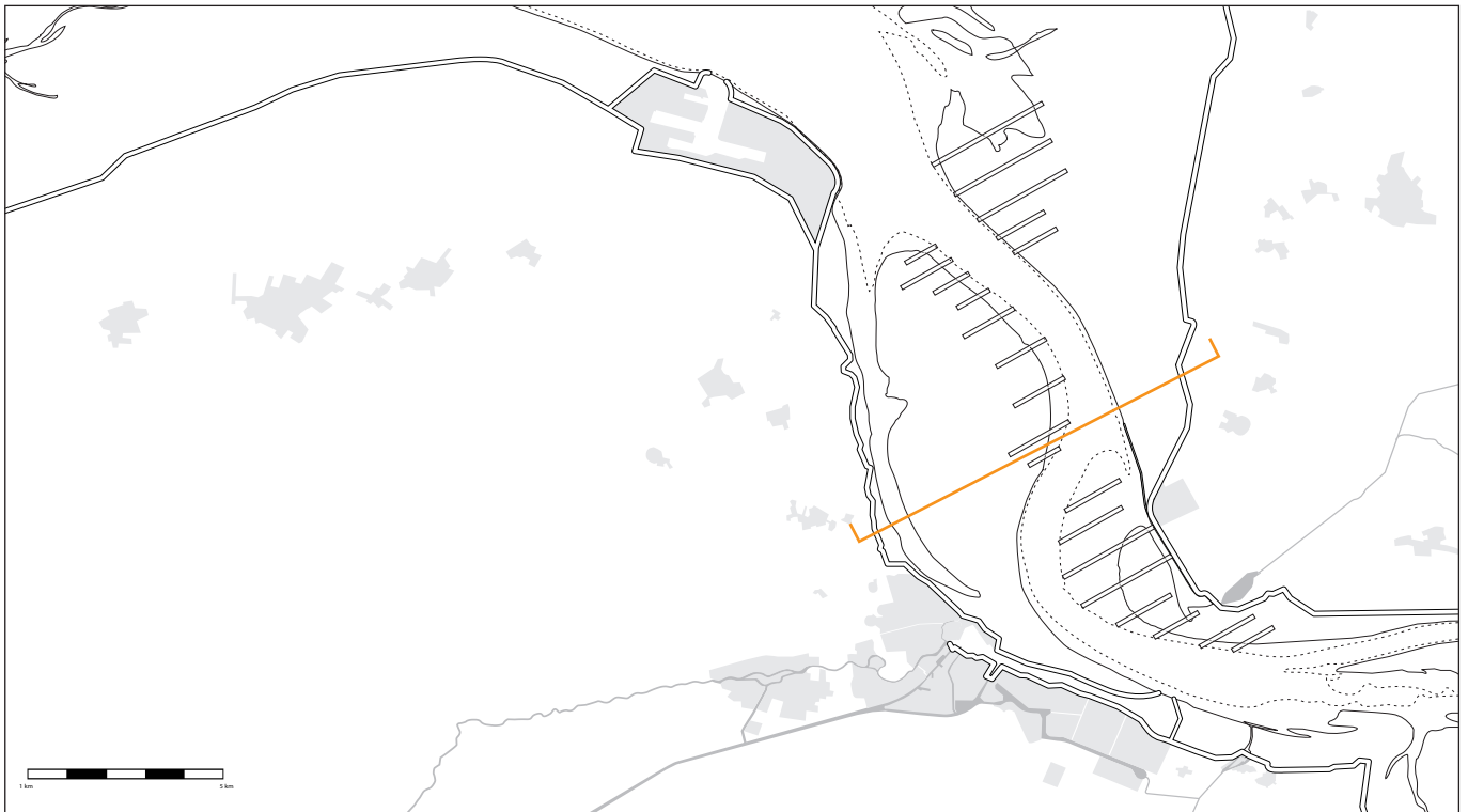
Figure 6.12(above) and 6.13(down) | Fase II. Extending the groynes ensures: a more intense meander, narrowing of the shipping channel and a broader side channel.
