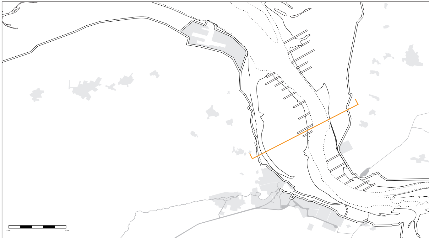
Figure 6.11 | Fase Ib. The water and thereby the course of the river searches a new course around the groynes.
