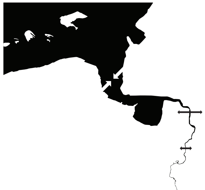
Figure 4.17 | Ems model To solve the Ems' turbidity problem the tidal inflow has to be limited at the estuarine mouth while the tidal basin has to be expanded in the tidal river zone.
