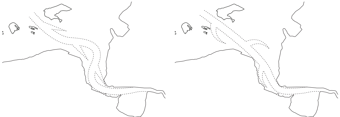
Figure 3.8 | Deformation of the multiple-channel system to a one-channel system (based on: Veen, 1950).
