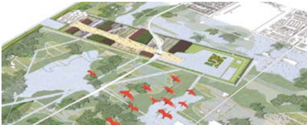
Figure 2.18 | Dredge landscape A landscape machine example. Polluted dredge is collected from rivers and canals in a single place in the Haarlemmermeer. The dredge is hence cleaned with natural processes, resulting in a park which grows and changes as the dredge is processed. (source: Herrebout & de Vries, 2006)
