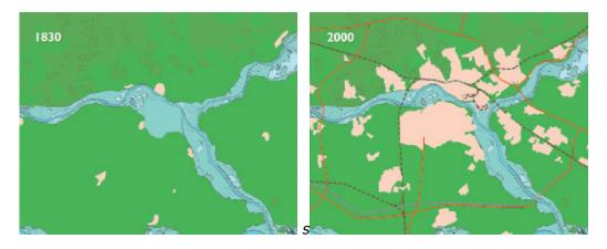
Figure 9: Reduction of the area of the flood plain at Arnhem between 1830 and 2000. More space was available to the river Rhine in 1926 than in 1995
