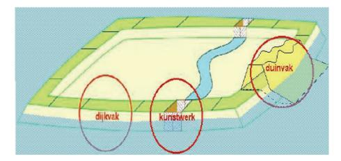
Figure 28: An enclosed continuous line of flood defenses composed of dike sections "dijkvak", dune sections "duinvak", structures "kunstwerk", and high ground (not shown).
