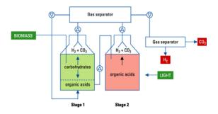
Figure 1: Two-stage bioprocess for hydrogen production from biomass
