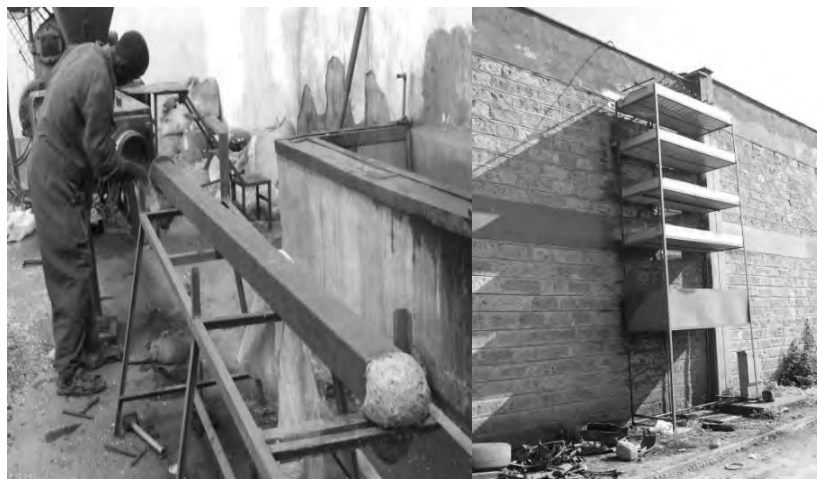
Photo Image 5-3 Extrusion of fencing post in a mould and water cooling system at Green Africa Limited (Photo by Bas van Vliet)
