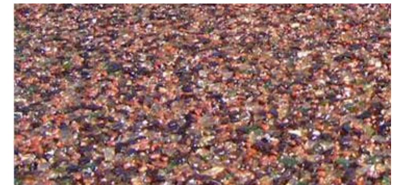
Figure 4.3.4 Close View on Filter Pave (Presto Geosystems, 2012)
