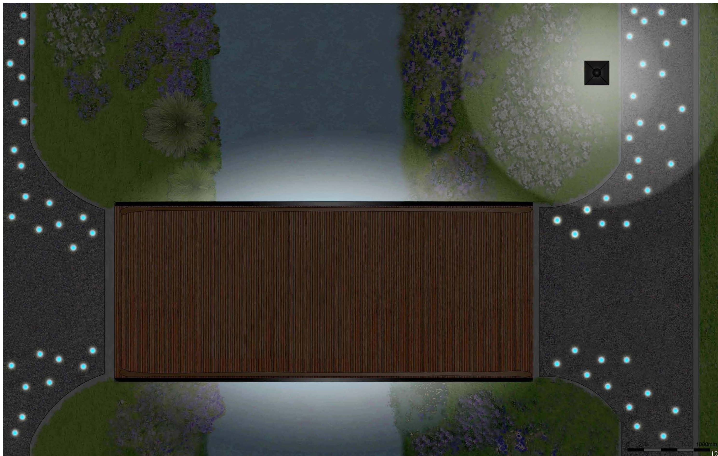
Figure 7.4.4 Detailed Design in Night Lighting: LED ground lights are flashing with blue light in the night to guide people to have nice brook experience with continuity.
