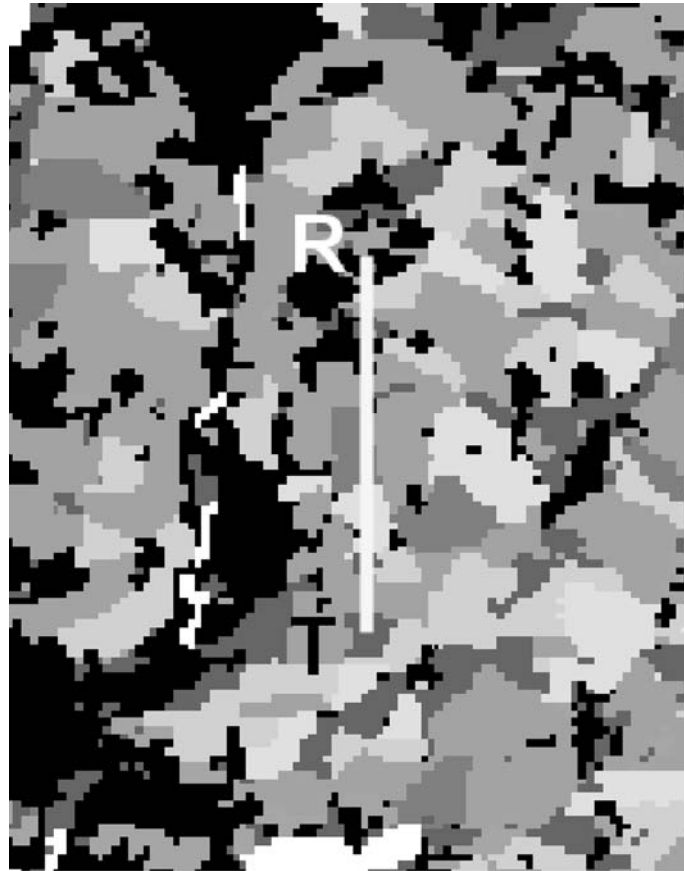
Figure 1. Eastern part of the LITFASS area ( 11 \times 8 \text{ km}^2 ) showing the source area of the LAS–MWS combination (white = open water; black = forest; dark grey = grass; medium grey = cereals; light grey = rape). The white line represents the path of the LAS–MWS, between the transmitter and receiver units, which are situated in Falkenberg (T) and Lindenberg (R), respectively.
