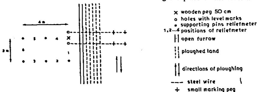
Beside each peg two holes are dug with a special auger, to a depth exceeding 10 cm the expected ploughing depth. The two holes are situated on a line parallel to the direction of ploughing and at a distance of 50 cm from the peg (FIG. 2). A level mark is placed on the bottom of each hole and tapped into a horizontal position.
