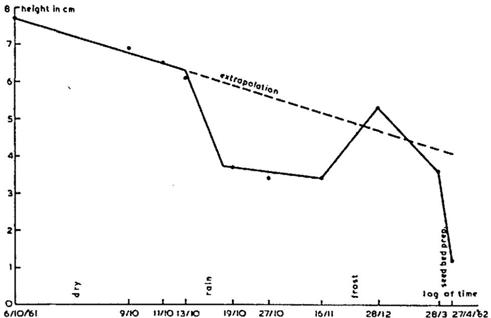
After this the rate of settling was so much slower, that the question arises whether the rains only changed the speed of the settling process and perhaps not the final state. Between the 16th of November and the 28th of December the soil surface rose at least about 2 cm by frost action. This rise did not entirely disappear in
