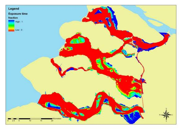
Figure 4.3 Calculated exposure time (fraction) scenario 3: connecting the basins.
