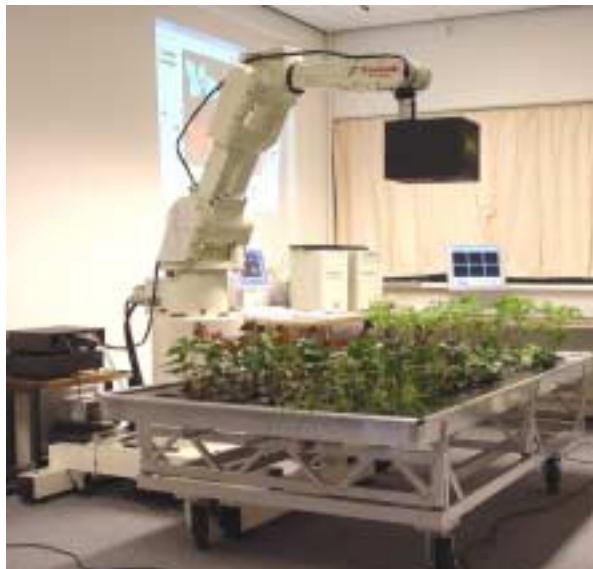
Figure 2. MIPS-Pro in action during the opening of the MIPS facility in 2002. The MIPS-Pro consists of a sensor head (black box) mounted on an industrial Kaawasaki robot. A plant table provides space for up to 85 petridishes.
