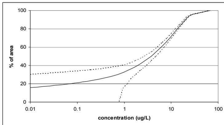
Figure 2 Cumulative distribution of leaching concentrations (µg/L) as calculated with the metamodel for the GeoPEARL schematization. Solid line: average value; dotted lines average ± standard deviation.
