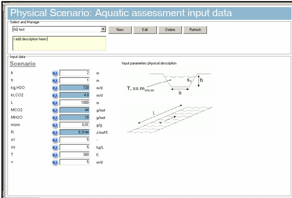
Figure 14. The Aquatic scenario input screen of PRIMET
