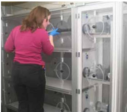
Odours are tested in an olfactometer.
