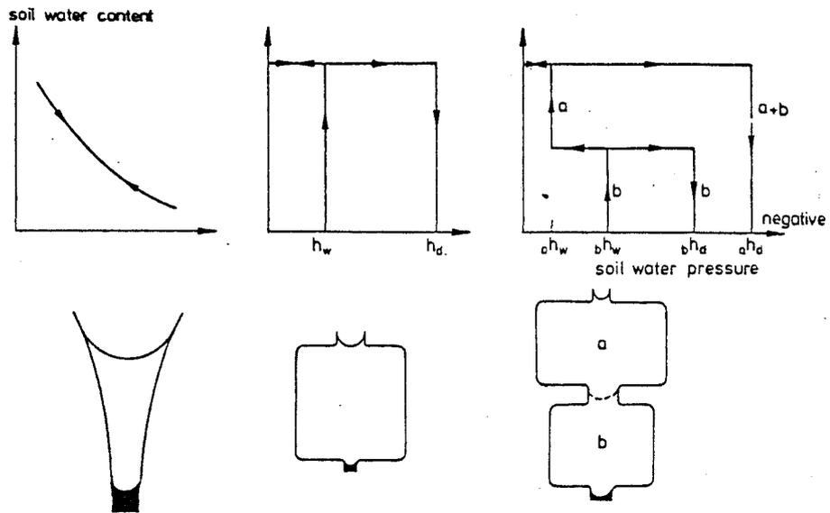
Fig. 2. Hysteretic effect of some pore configurations on water retention curve (after POULOVASSILIS, 1962)
