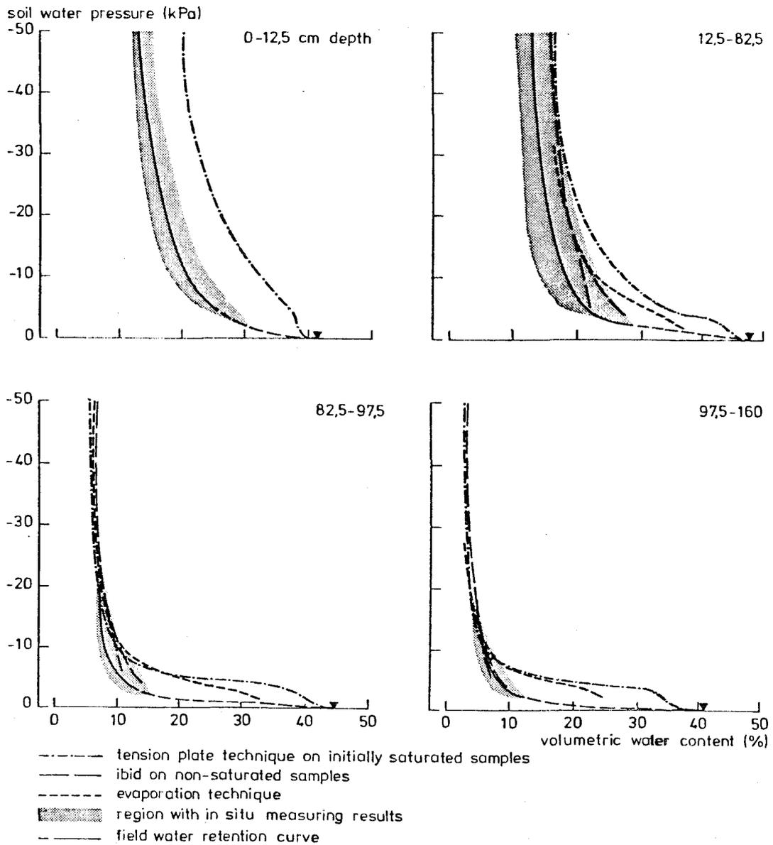
Fig. 11. Water retentivity of different soil layers at the experimental field, measured in situ and in the laboratory
