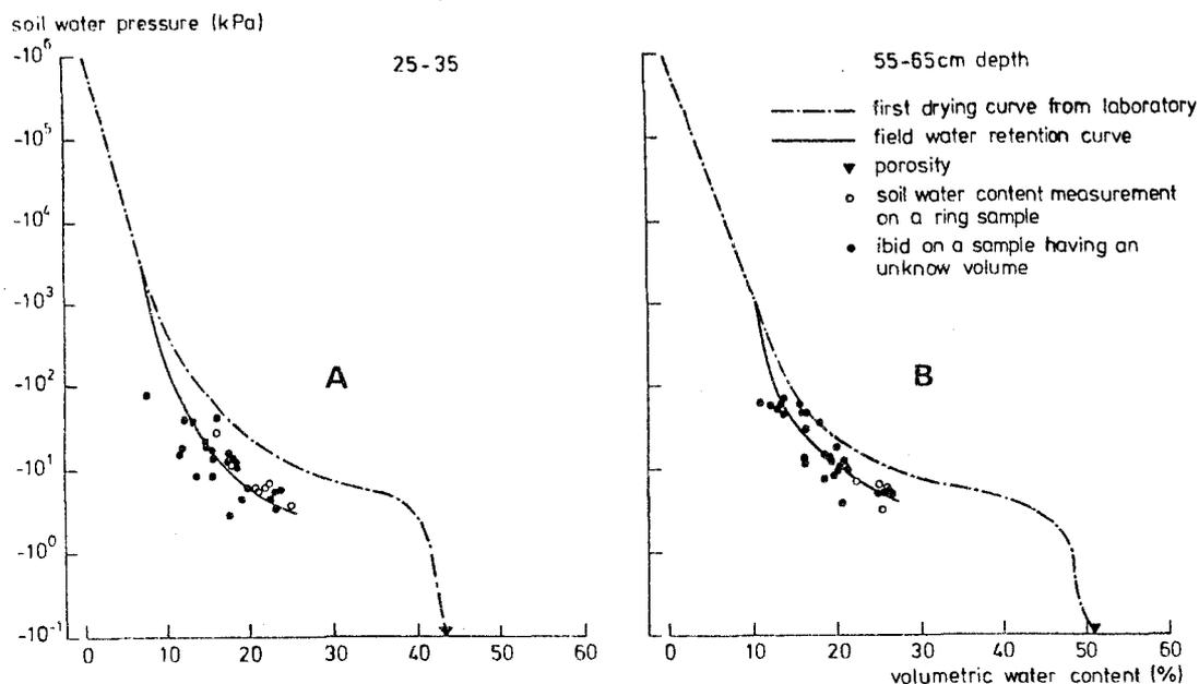
Fig. 13. Water retentivity measured in situ at two levels in the soil at the experimental field
