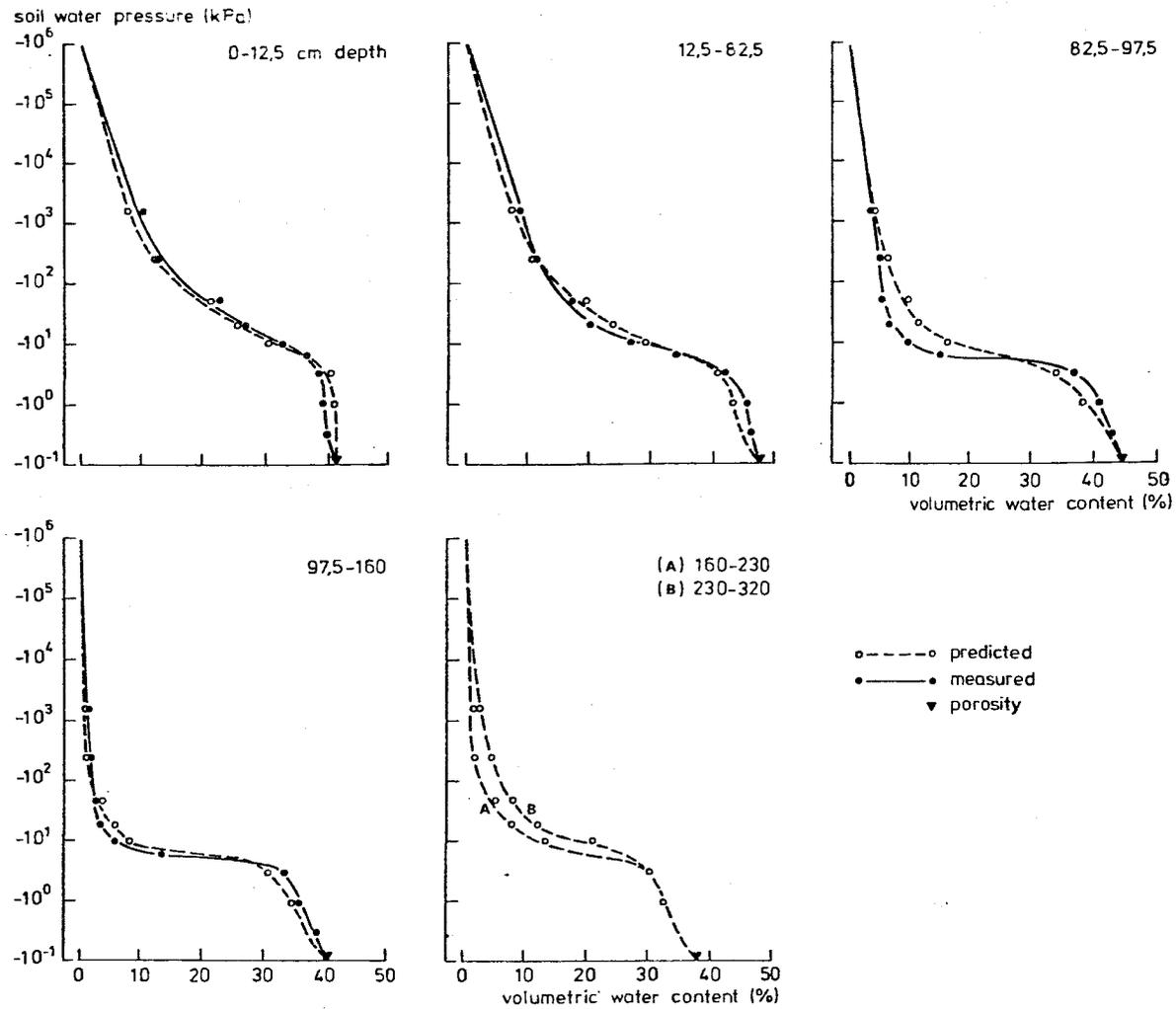
Fig. 10. Predicted and measured results of pressure cell and tension plate methods on initially saturated soil samples from the experimental field
