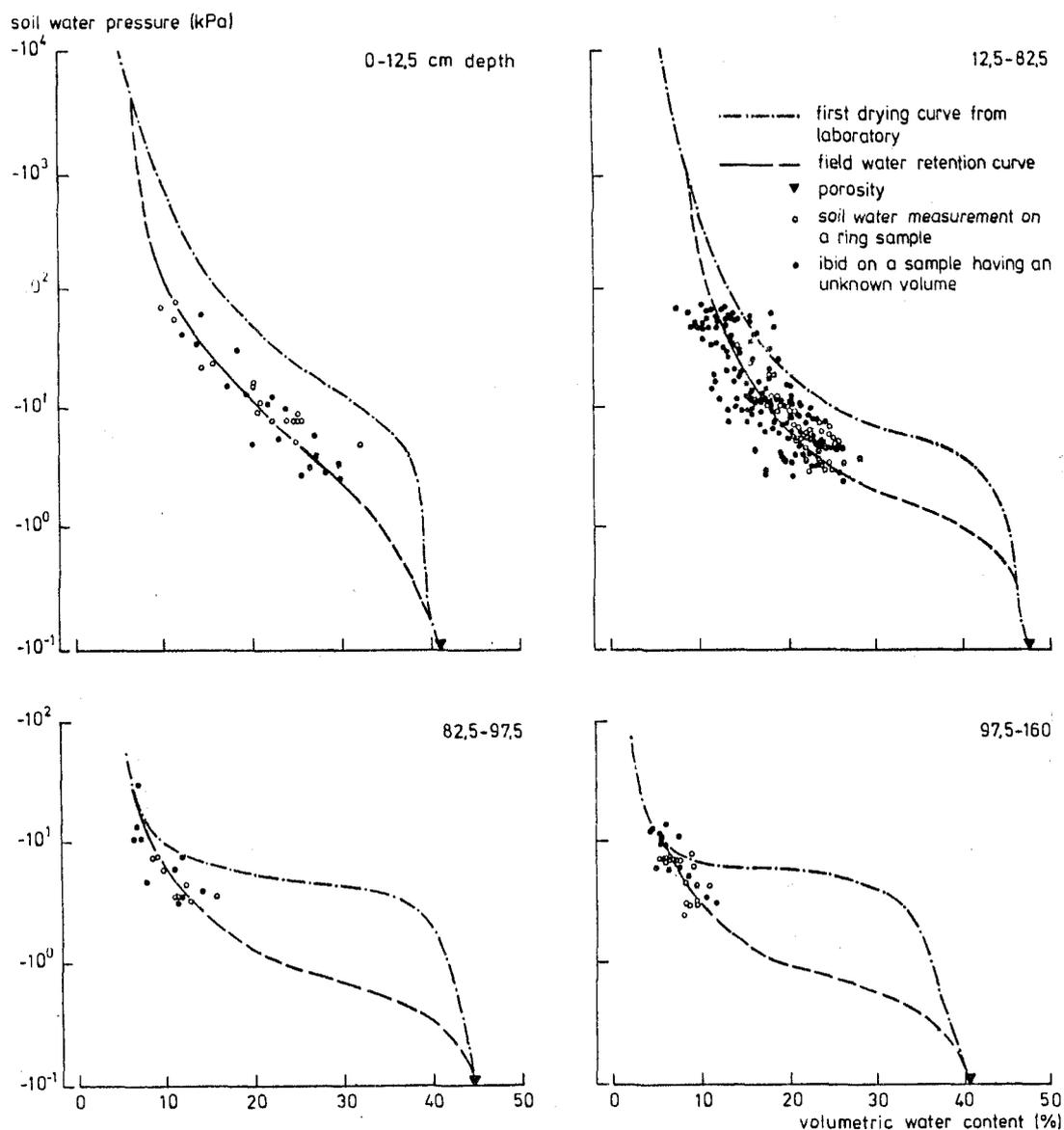
Fig. 12. Water retentivity of different soil layers at the experimental field, according to in situ measuring results
