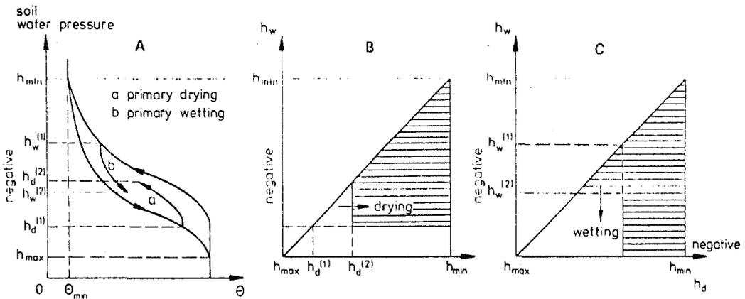
Fig. 6. A. a primary drying and primary wetting scanning curve, B. primary drying process; the elements with  $h_d, h_w$ -values in the arced region will be drained out, C. primary wetting process; the elements with  $h_d, h_w$ -values in the arced region have been re-entered
