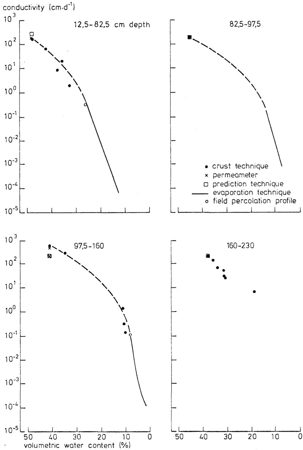
Fig. 16. Hydraulic conductivity of different soil layers at the experimental field
