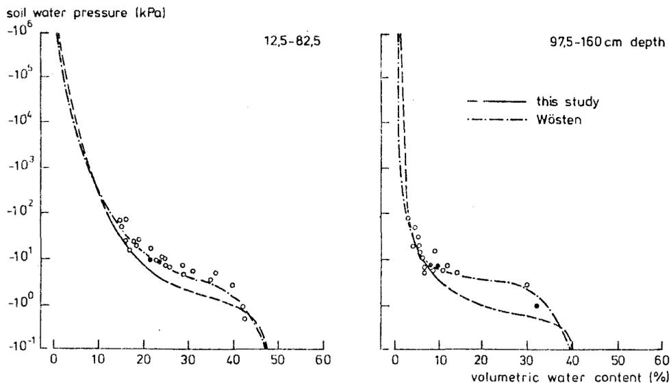
Fig. 14. Water retention curves derived by WOSTEN (1983) from laboratory (o) and in situ (●) measurements on samples from the layers 12.5-82.5 and 97.5-160 cm below surface, as well as the corresponding curves derived in this study from in situ measurements
