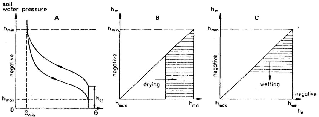
Fig. 5. A. a main drying and main wetting curve, B. main drying process; the elements with  $h_d, h_w$ -values in the arced region will be drained out, C. main wetting process; the elements with  $h_d, h_w$ -values in the arced region have been re-entered
