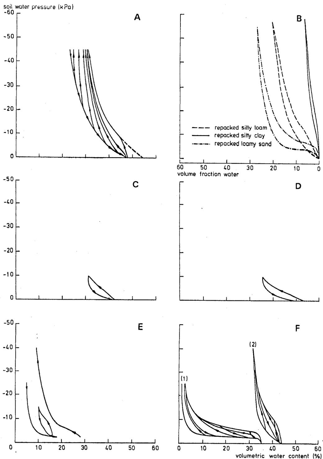
Fig. 3. Hysteretic water retention curves found in literature. A. repacked silt loam, after STAPLE (1966); B. after CARY (1975); C. undisturbed sand with 5 percent organic matter and density of  $1.47 \text{ t}\cdot\text{m}^{-3}$ , after ILNICKI (1982); D. ibid with 9 percent organic matter and density of  $1.14 \text{ t}\cdot\text{m}^{-3}$ , after ILNICKI (1982); E. in situ fine sand, after ROYER and VACHAUD (1975); F. in situ loess (1) and gravelly sand (2), after RENGGER et al. (1974)
