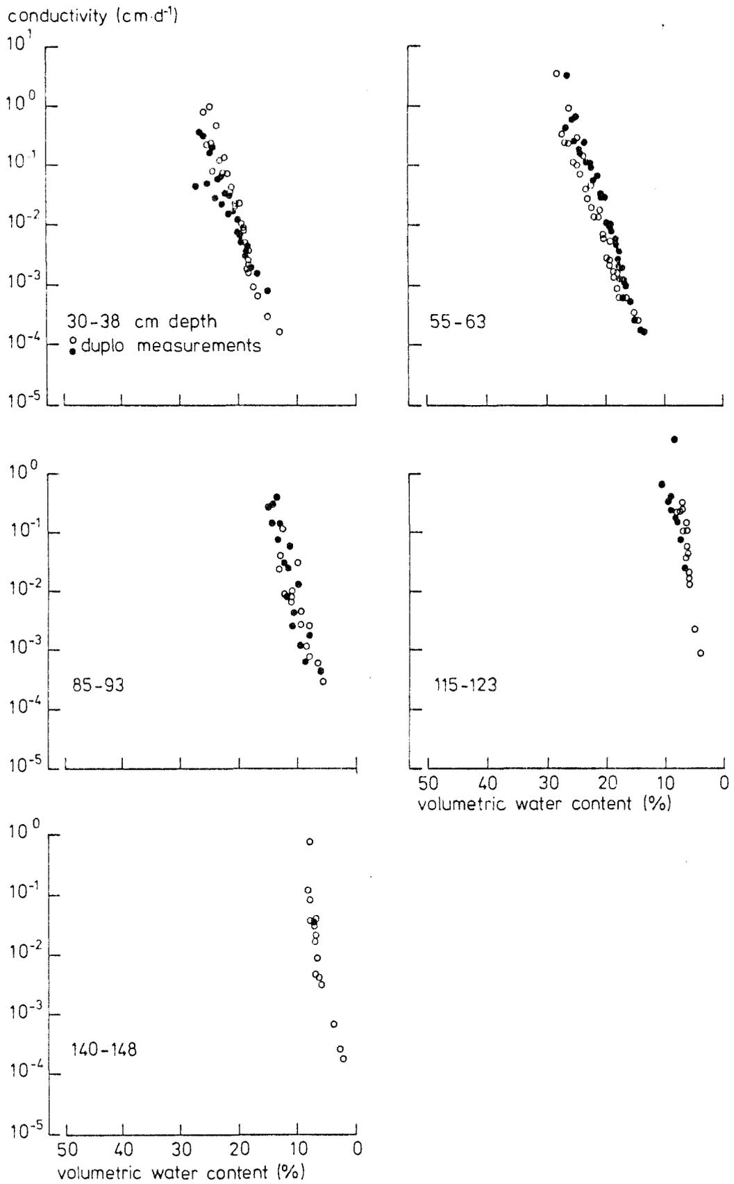
Fig. 15. Hydraulic conductivity of different soil samples from the experimental field measured according to the evaporation technique of BOELS et al. (1978)
