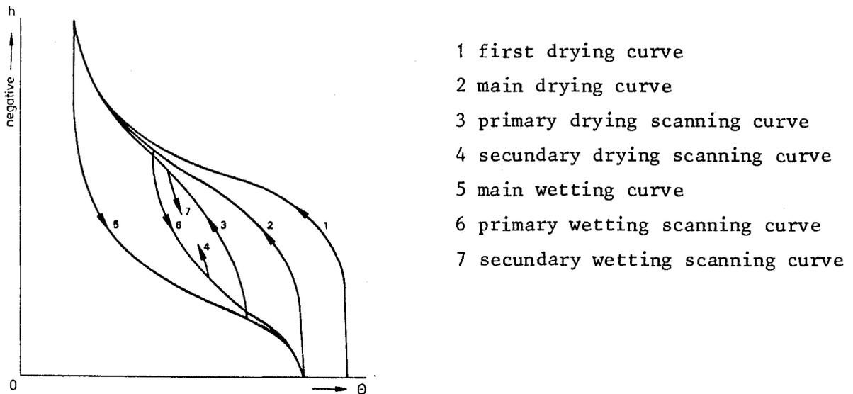
Fig. 1. Hysteretic relationships between soil water pressure  $h$  and soil water content  $\theta$
