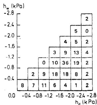
Fig. 7. Domain diagram determined for a glass-bead structure, showing the volumes of the elements ( $\text{cm}^3$ ) draining out and re-entering the medium of different water pressure ranges within the main hysteresis loop (after POULOVASSILIS, 1962)
