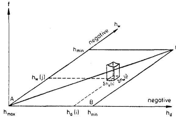
Fig. 4. Graphical presentation of volume  $f$  corresponding to the soil water element draining out of the soil at water pressure change  $\delta h_d(i)$  and re-entering at water pressure change  $\delta h_w(j)$  (after POULOVASSILIS, 1962)
