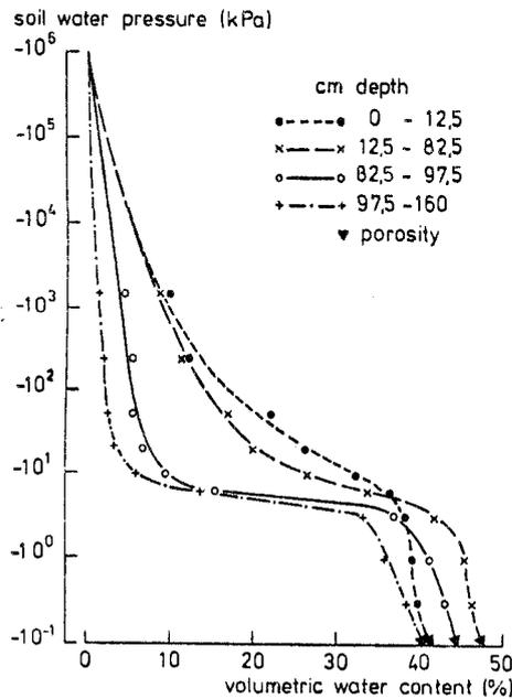
Fig. 9. Water retention curves derived from pressure cell and tension plate measurements on initially saturated soil samples from the experimental field
