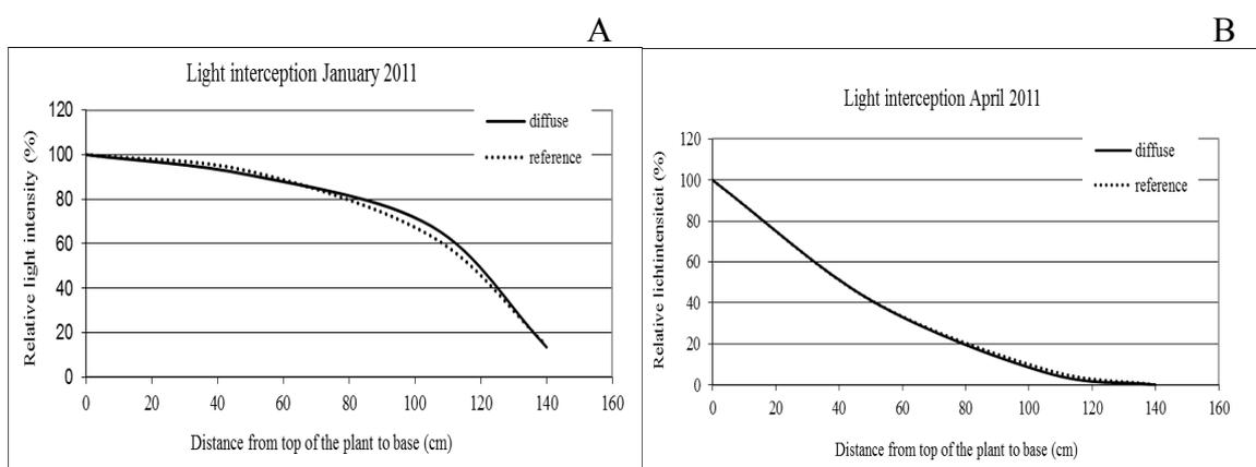
Fig. 4. Light interception by the crop at different heights in both greenhouses. A: situation in January; B: situation in April.
