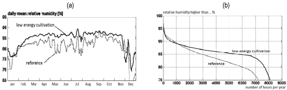
Fig. 2. The effect of the low energy cultivation on daily mean relative humidity and on the number of hours per year where humidity is above a certain threshold value.
