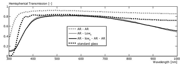
Fig. 3. Optical properties of the double greenhouse glass used. Spectral hemispherical light transmission of single glass with two anti-reflection coatings (AR-AR), single glass with one anti-reflection and one low-emission coating (AR-Low e) and double glass consisting of the two types of single glasses (AR-Low e-AR-AR) compared to a single reference glass.
