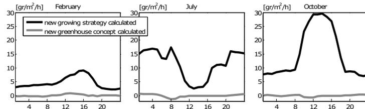
Fig. 7. Dehumidification by condensation at the inner surface of the greenhouse covering calculated for typical months.
