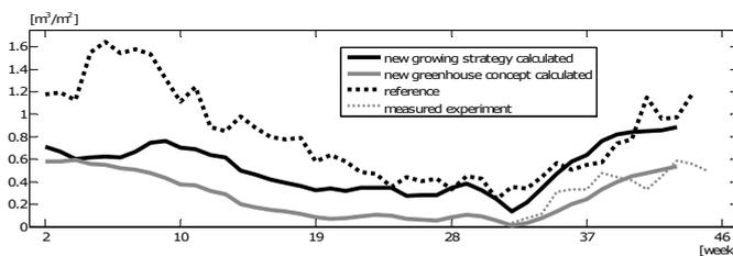
Fig. 4. Calculated (year-round) and realised (week 32 until 45) energy consumption in a cucumber crop for three different scenarios: Reference (traditional greenhouse, climate control like horticultural practice), New growing strategy (traditional greenhouse, new climate control strategy), New greenhouse concept (double glass with new climate control strategy).
