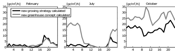
Fig. 6. Dehumidification by the mechanical system calculated for typical months.
