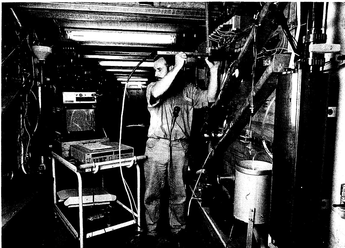
Fig. 6. Underground corridor with instrumentation, irrigation tanks and access ports of minirhizotrons during recording of rooting patterns using the videocamera.
