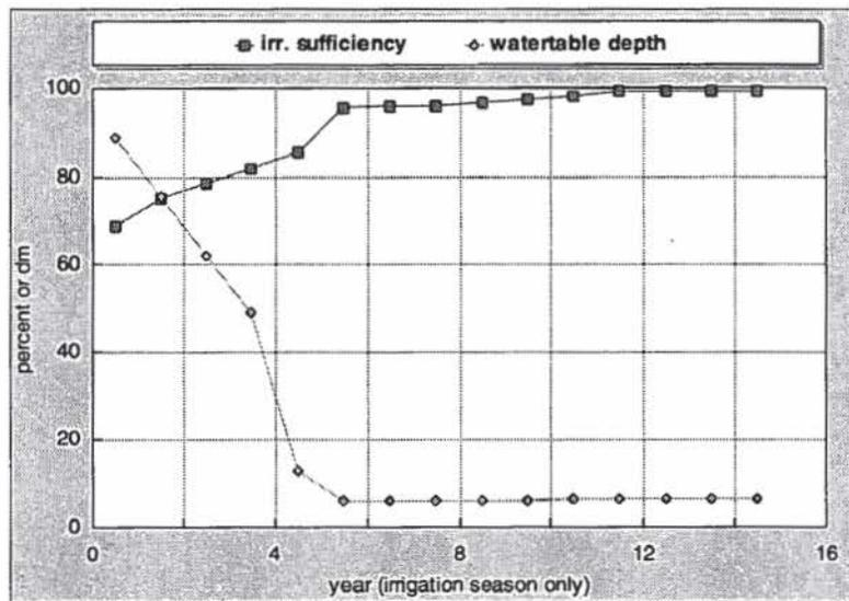
**Figure 2. Effects of watertable depth on irrigation sufficiency**
