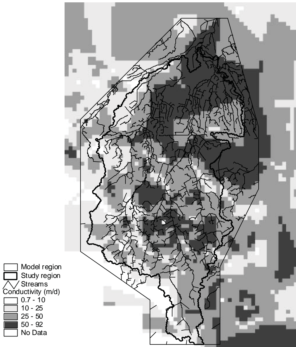
Figure 3.3 Example of a map of the subsoil conductivity, provided by NITG-TNO through the REGIS-database for the 'Sterksel/Nuenen coarse' layer (layer 3, Tabel 3.1)
