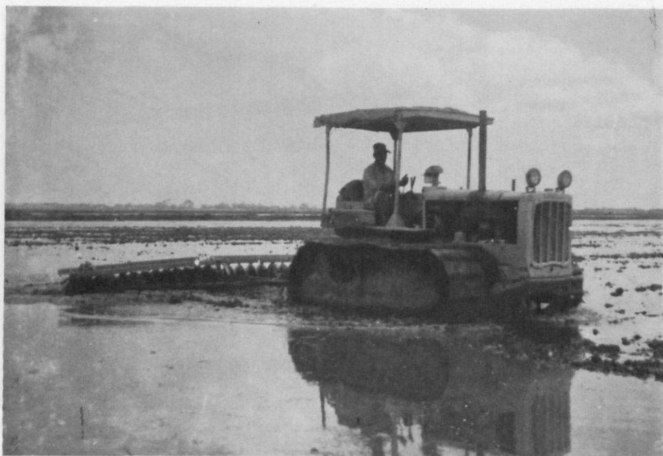
Photo 12. Puddling with a John Deere single disc harrow.
