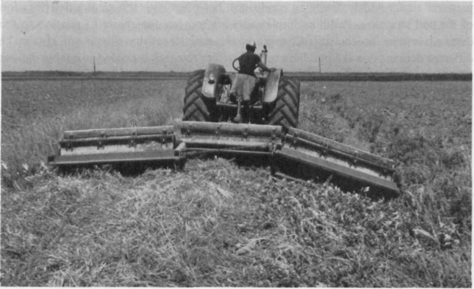
Photo 8. Cutting the vegetation on dams with a Marden T-5 weed-cutter.
