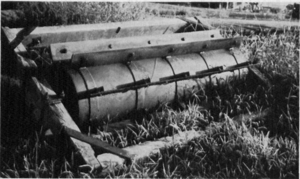
Photo 9. A closed roller with steel knives used in the Prince Bernhard Polder.
