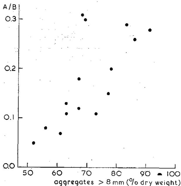
FIG. 2. THE RATIO (MOISTURE PERCENTAGE AT pF 1.9 MINUS LOWER PLASTIC LIMIT) : (sticky point minus moisture percentage at pF 1.9) as related to the percentage aggregates > 8 mm in a marine clay soil (Pr 842).
