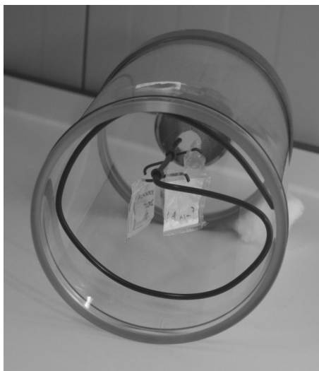
Figure 7.7. LDPE sachets used to test synthetic compounds.
