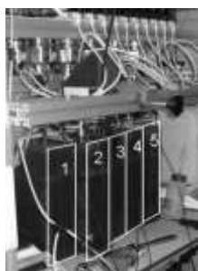
Figure 2 - Vessels used for the shear test and to determine sludge filterability.
