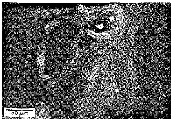
Fig. 34. Floc structure of the activated sludge under the phase-contrast microscope. The sludge was grown in the chemostat fed on vanillin (Section 4.2.1) where \mu = 0.032 \text{ h}^{-1} .
