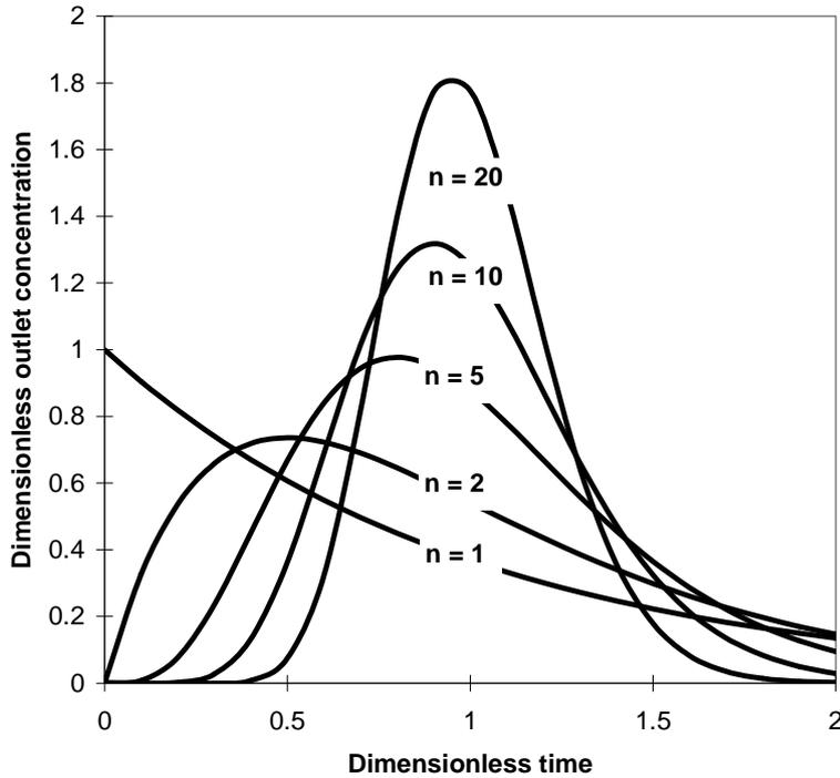
Figure 5-10(L2) Effect of number of CSTRs,  $n$ , on a tracer added instantaneously to the inlet of a tank. Note: dimensionless time = 1 is equivalent to the HRT of the tank
