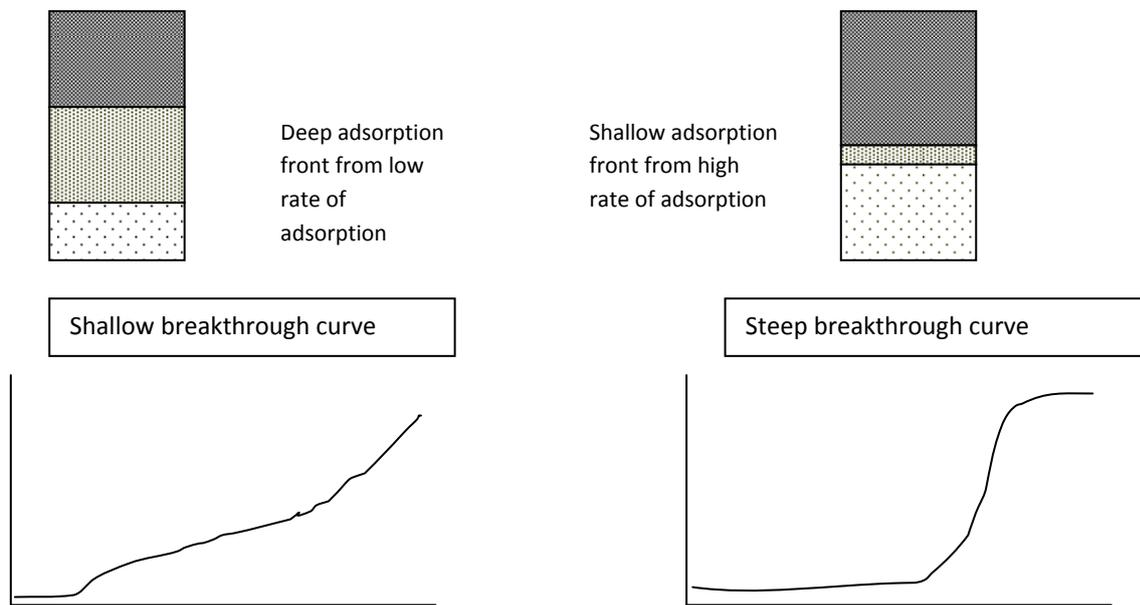
Figure 5-3 Effect of the adsorption front on the shape of the breakthrough curve
