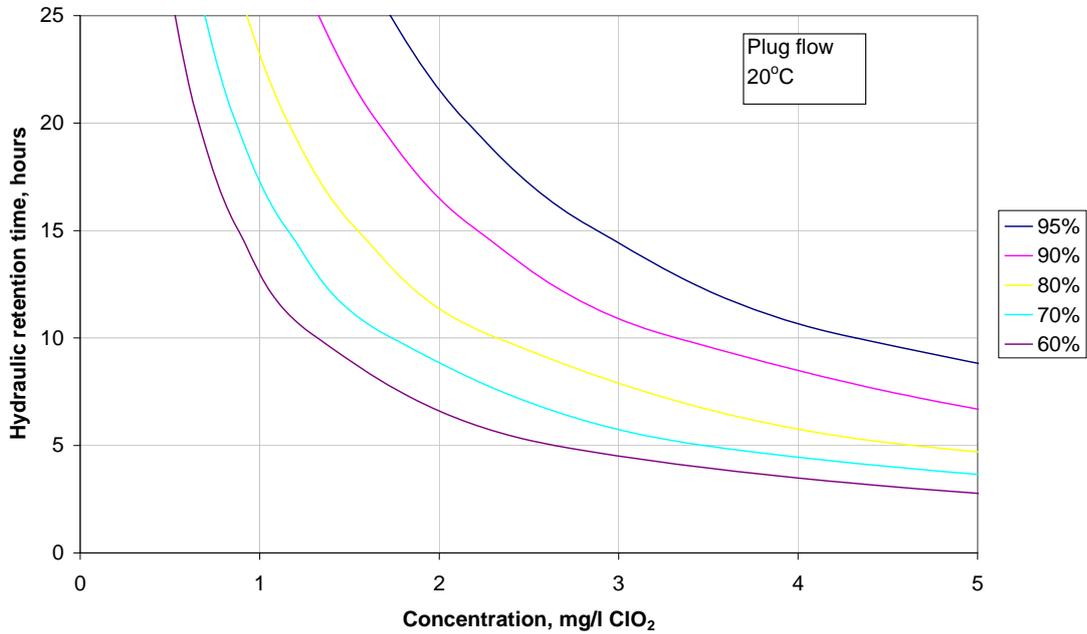
Figure 5-15(L2) Performance of chlorine dioxide for m-LR breakdown
