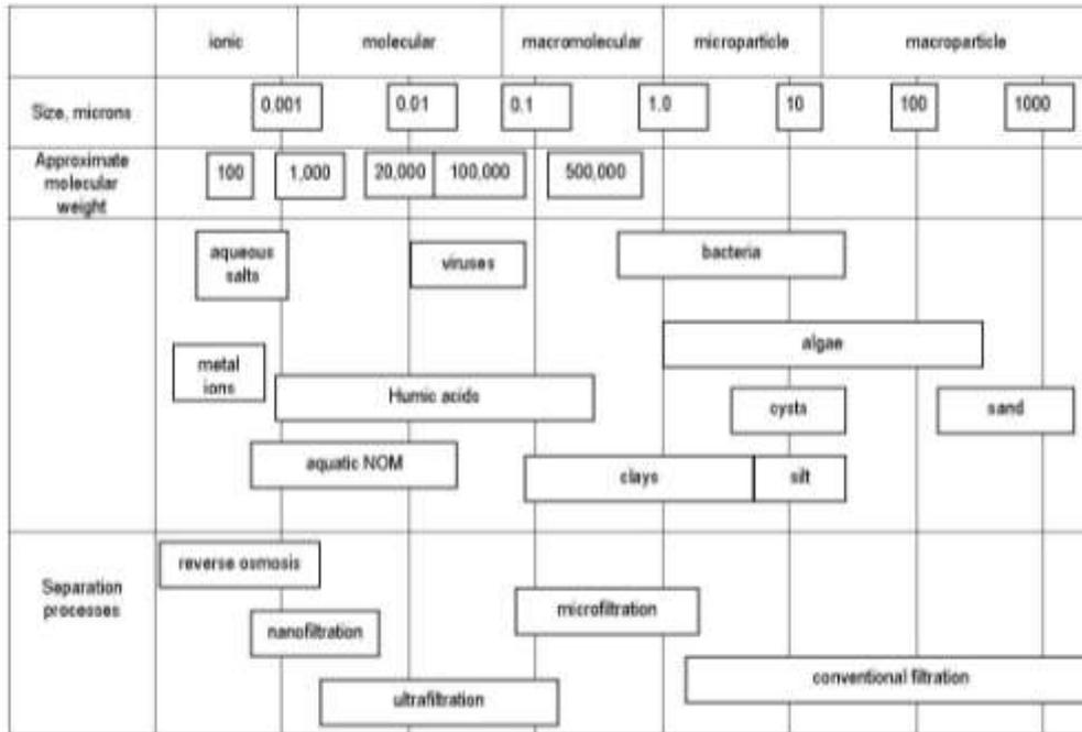
Figure 5-2 Efficiency of various filtration processes
