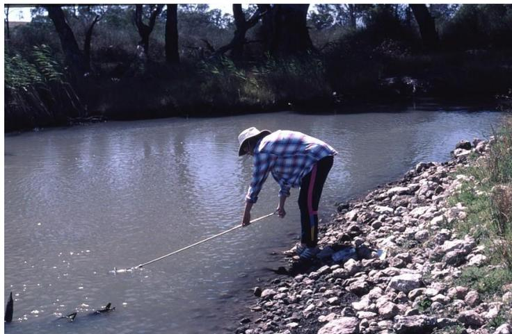
Figure 3-4 Taking grab samples from the shoreline with an extension pole.
