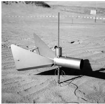
Figure 7 Two examples of equipment that the Land Degradation and Development Group developed together with Royal Eijkelpkamp. Left, a mini rainfall simulator for use in remote areas. Right, the saltiphone that detects the flow of saltation particles in wind erosion.
