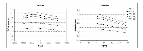
Figure 5: Load safety factor for variations of hurricane parameters
