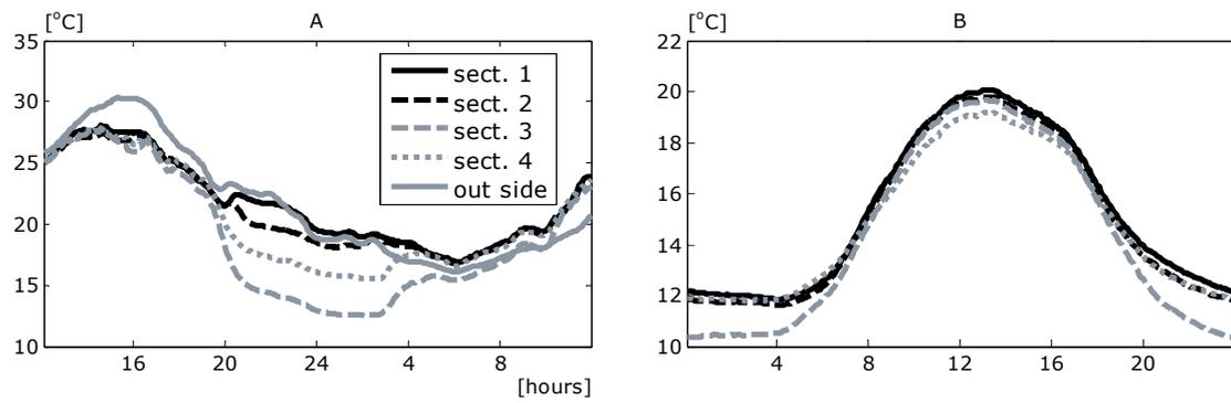
Fig. 3. Outside and greenhouse air temperature in four sections from August 24<sup>th</sup> 12:00 till August 25<sup>th</sup> 12:00 (A) and twenty four hours average of greenhouse air temperature in the four sections from August 11<sup>th</sup> till January 5<sup>th</sup> (B).
