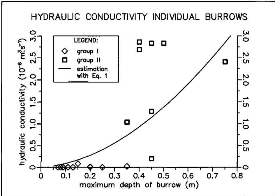
Fig. 7.2 Measured and estimated (Eq. 7.1) saturated hydraulic conductivity of individual surface open burrows,  $K_b$  ( $\text{m}^3 \cdot \text{s}^{-1}$ ), in relation with their maximum obtained depth,  $z_b$  (m). Group I, low conductivity ( $\leq 10^{-7} \text{ m}^3 \cdot \text{s}^{-1}$ ), group II high conductivity ( $> 10^{-7} \text{ m}^3 \cdot \text{s}^{-1}$ ).
