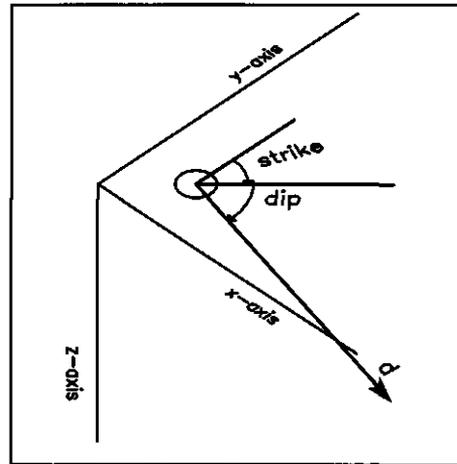
Figure 2.2 Dip and strike for a burrow with direction  $d$ . The burrow is depicted as a horizontal circle.
