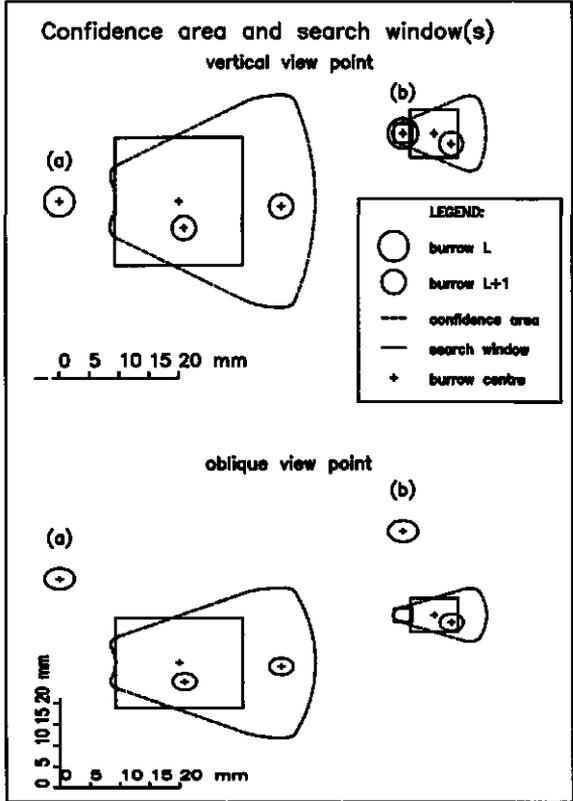
Figure 2.4. (Top) Search window(s) and confidence area for a burrow with (a) a dip of 31-60° and (b) a dip of 61-90°. The direction of view is perpendicular to the horizontal plane. (Bottom) Search window(s) and confidence area for a burrow with (a) a dip of 31-60° and (b) a dip of 61-90°. The direction of view makes an angle of 45° with the horizontal plane.
