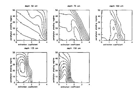
Fig. 9.24. Nomograms showing the effect of constant periphyton shading regime and constant water layer extinction coefficient on peak tuber biomass in the 10th simulation year for various water depths.
