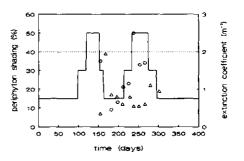
Fig. 9.5. Periphyton shading regime (solid line) and water layer light extinction (dotted line), as used during model calibration ('Lake Veluwe conditions'). The actually measured periphyton shading percentages during 1986 (triangles) and 1987 (circles) under unshaded conditions in Lake Veluwe are shown also.
