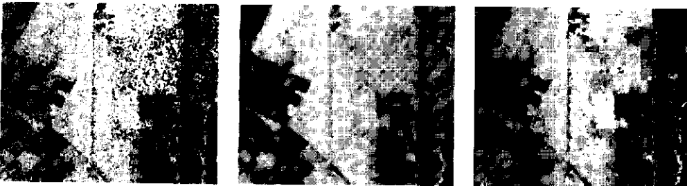
Figure 6.2 (a-c). Seasat image of the Roggebotzand recorded on 28 August 1978: (a) unprocessed image, (b) result of median filter with 5 x 5 pixel window, (c) result of split-and-merge segmentation.
