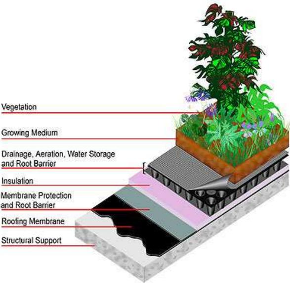
Figure 5.2: Typical layers of the intensive and extensive roof type (Garmann/Miller, 2008)
