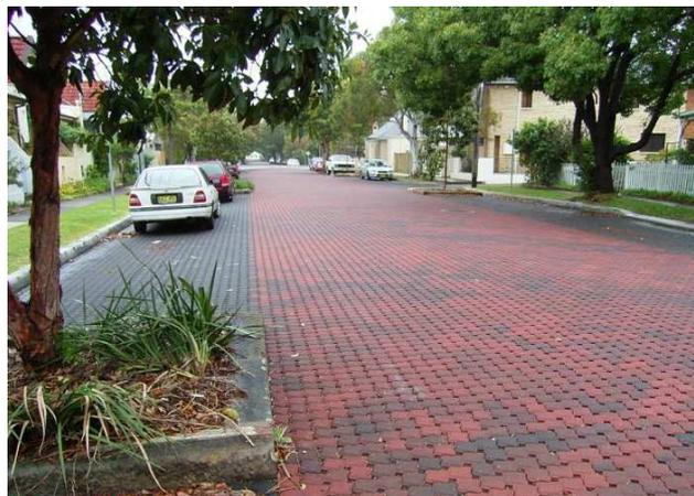
Figure 5.7: *Example of a permeable road (North Coast Stormwater Coalition, 2010)*
