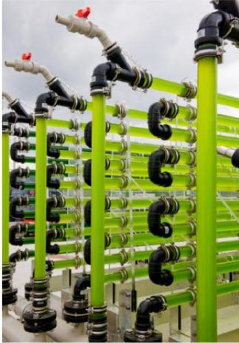
Figure 16 Picture of a vertical tubular PBR (Wolkers et al., 2011)
