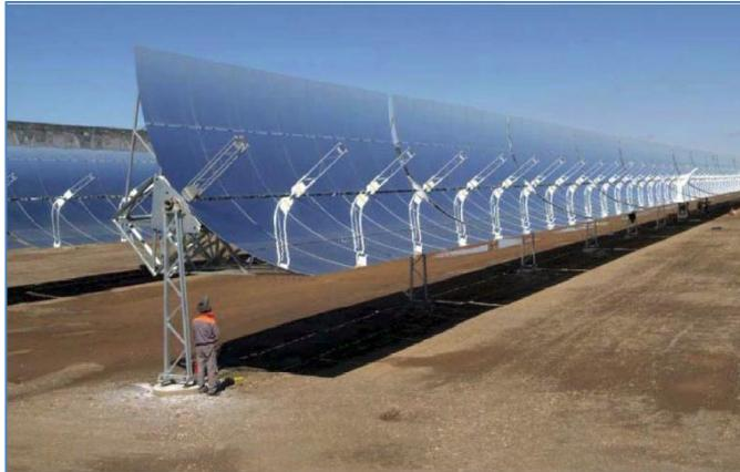
Figure 6 Parabolic trough type solar collector (from [www.solarserver.com/knowledge/basicknowledge/solar-collectors](http://www.solarserver.com/knowledge/basicknowledge/solar-collectors)).
