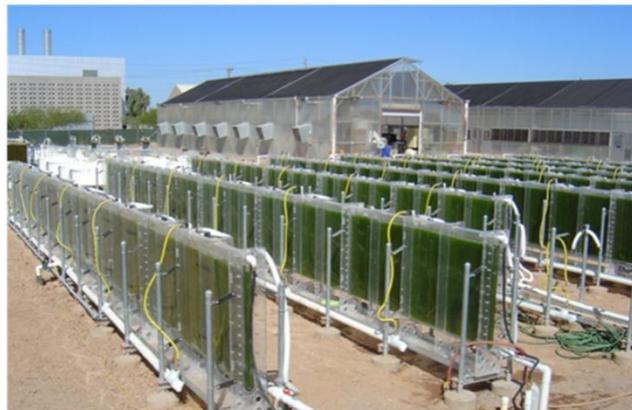
Figure 17 Picture of a flat plate PBR (<http://www.cleantick.com/users/franc/pages/developments-in-closed-reactors-for-algae-cultivation/updates/10245>)
