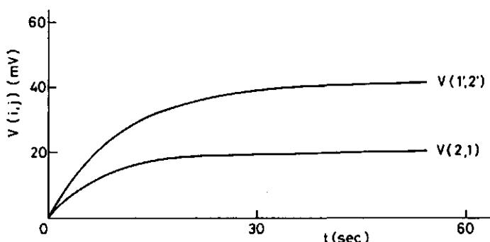
Fig. 3.14 - Polarization of Pt black electrodes during streaming current measurements (plug II, 7 \times 10^{-4} M KCL, \Delta P = 30 cm Hg).
