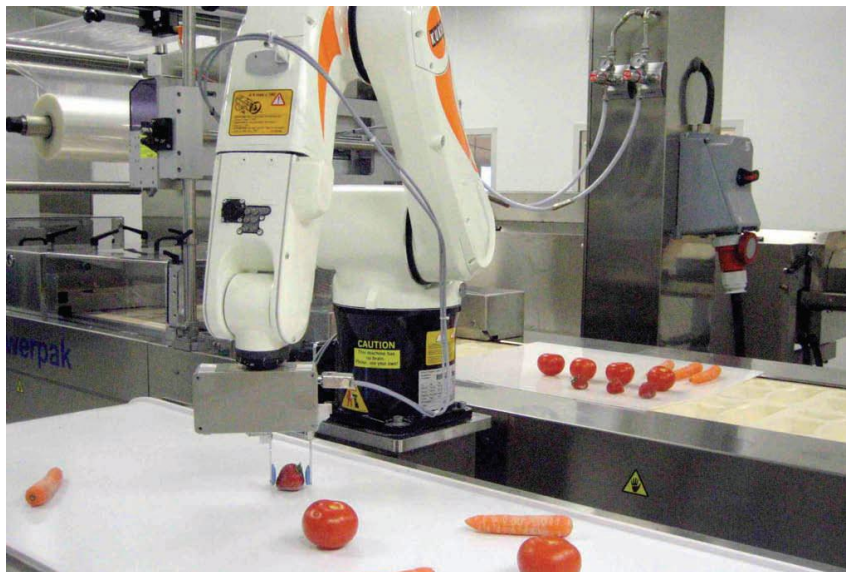
Figure 2.4.1 Robot station during flexible production. Variable and fragile products arrive mixed to the robot and are individually handled and placed according to the layout designed.
