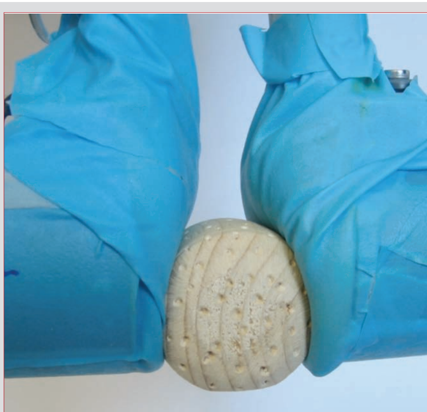
Figure 2 MR-fluid gripper arms holding a wooden model of a strawberry
