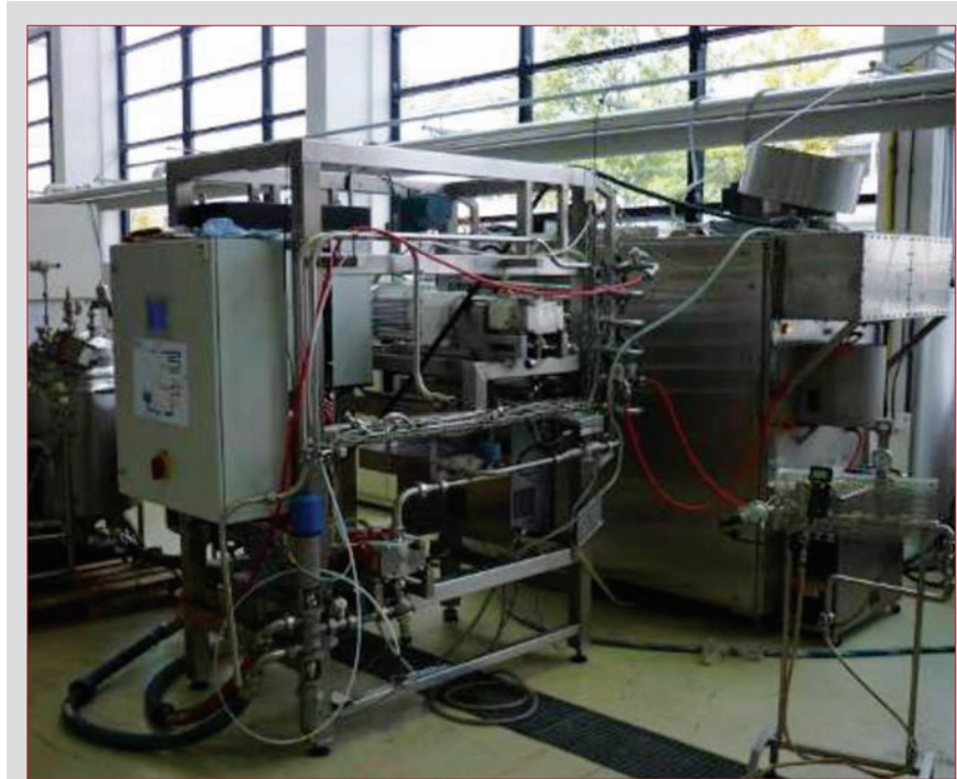
Figure 3 Pilot-scale pulsed electric field equipment including pre and post handling for trials with pumpable food products (pilot PEF unit Wageningen UR)
