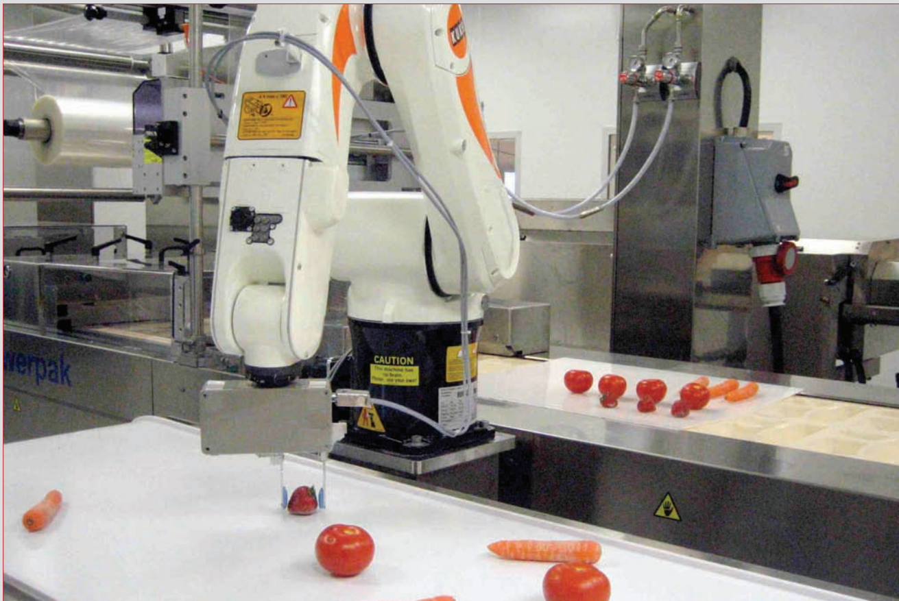
Figure 5 Robot station during flexible production. Variable and fragile products arrive mixed to the robot and are individually handled and placed according to the layout designed in the GUI
