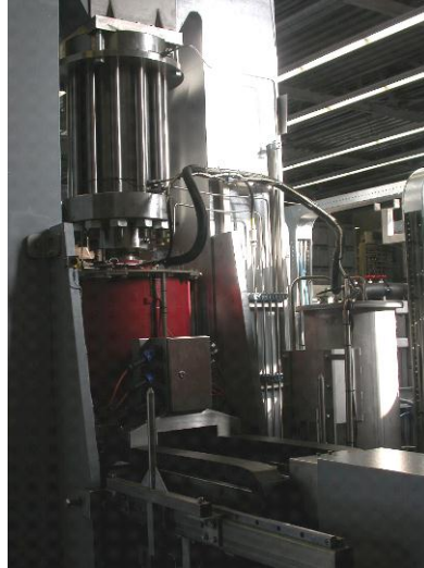
Figure 2.4.5 Part of a high pressure sterilisation unit where sealing is essential at the high pressure vessel and the intensifier used to achieve the high pressure necessary for sterilisation.
