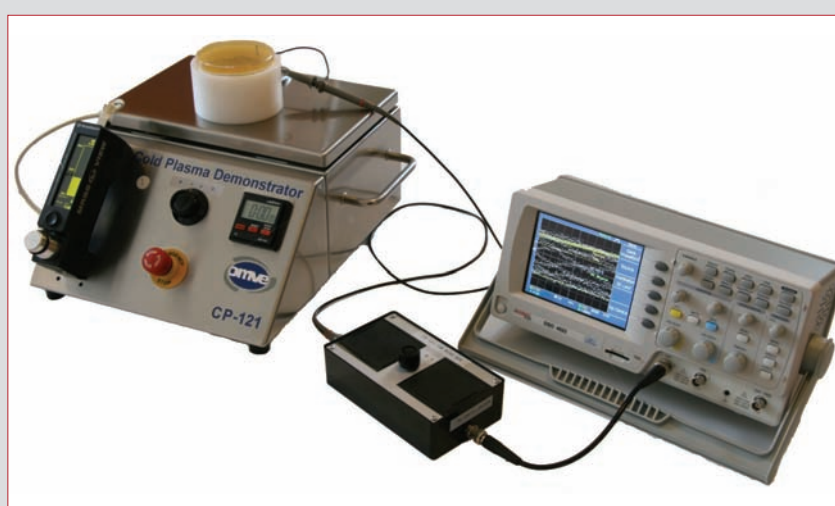
Figure 5 A laboratory scale cold plasma unit including diagnostics that was developed by Wageningen UR Food & Biobased Research developed in collaboration with the Dutch SME OMVE BV
