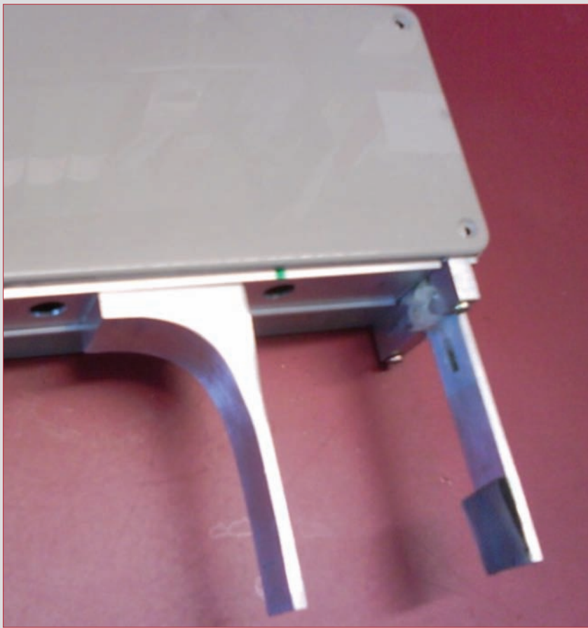
Figure 3 Enclosed parallel arm gripper actuator with force sensor and magnetic coupling. The base of the moving arm (left) contains the set of magnets
