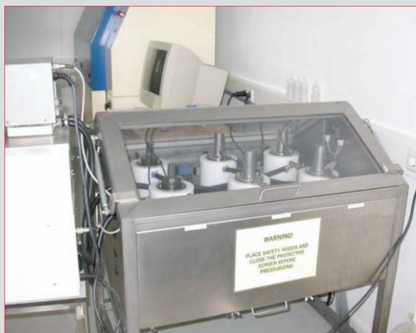
Figure 2 Characteristic lab-scale HP equipment for inactivation kinetics (multi-vessel system, Wageningen UR)
