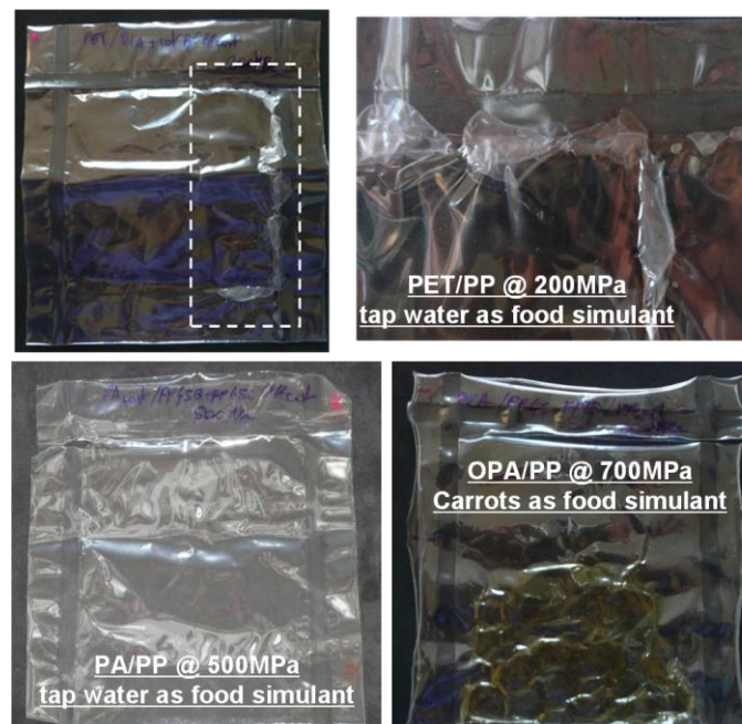
Figure 2.2.3 Examples of multilayers films subjected to HP sterilization: i) delamination occurring after HP sterilization in PET/PP bilayers and ii) structural integrity after HP sterilization in PA/PP and OPA/PP bilayers. PP: Unoriented Polypropylene; OPA: Biaxially oriented polyamide; PA: Unoriented polyamide
