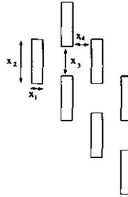
Figure 5.3: Parametrization of the slot grid pattern
