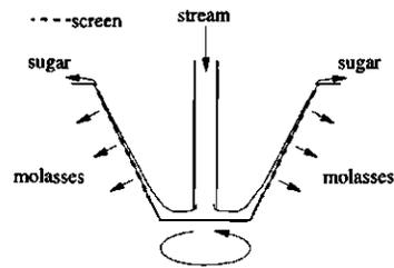
Figure 5.2: Continuous sugar centrifugal
