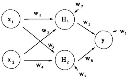
Figure 2.8: Small neural net with two inputs, one output and two hidden nodes
