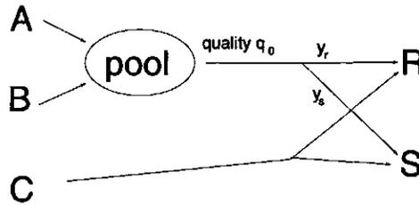
Figure 2.6: Blending with combined storage, the Haverly pooling problem
