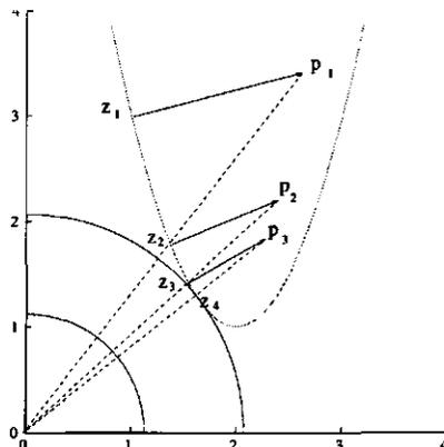
Figure 4.21: Algorithm for solving the maximum sphere problem, quadratic properties
