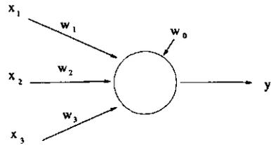
Figure 2.7: One node of a neural net
