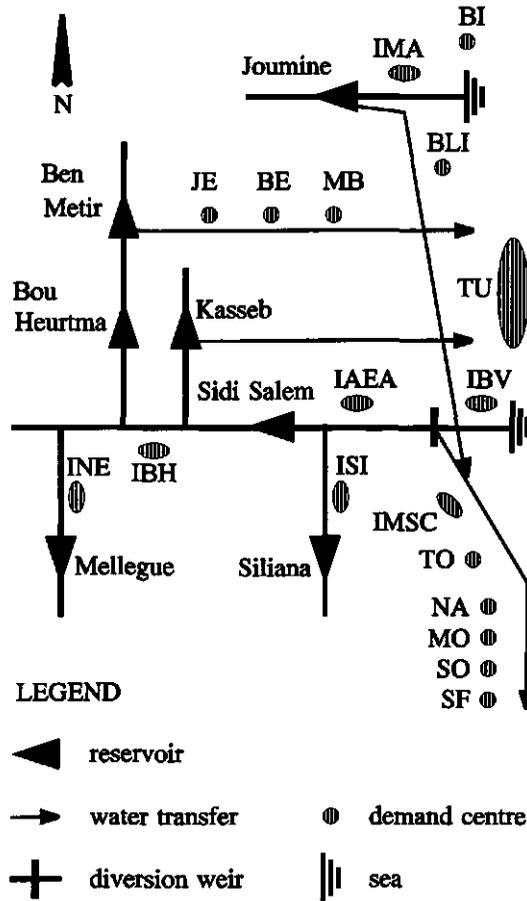
Figure 5.5: Seven reservoir system in Tunisia. Source: Milutin and Bogardi, 1996
