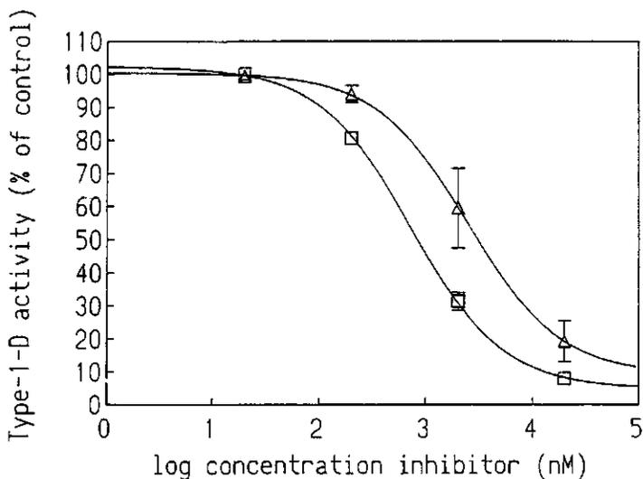
Figure 4 Inhibition of ID-1 activity by the hydroxylated PCB metabolites of 5-OH-3,3',4,4'-tetraCB (F,  $\Delta$ ) and 4,4'-(OH)<sub>2</sub>-3,3',5,5'-tetraCB (J,  $\square$ ). Datapoints are mean values of triplicates with standard deviation. Control ID-1 activity was  $60.45$  pmol l/min/mg. Percentage of ID-1 inhibition compared to control is plotted against log concentration of competitor (nM).
