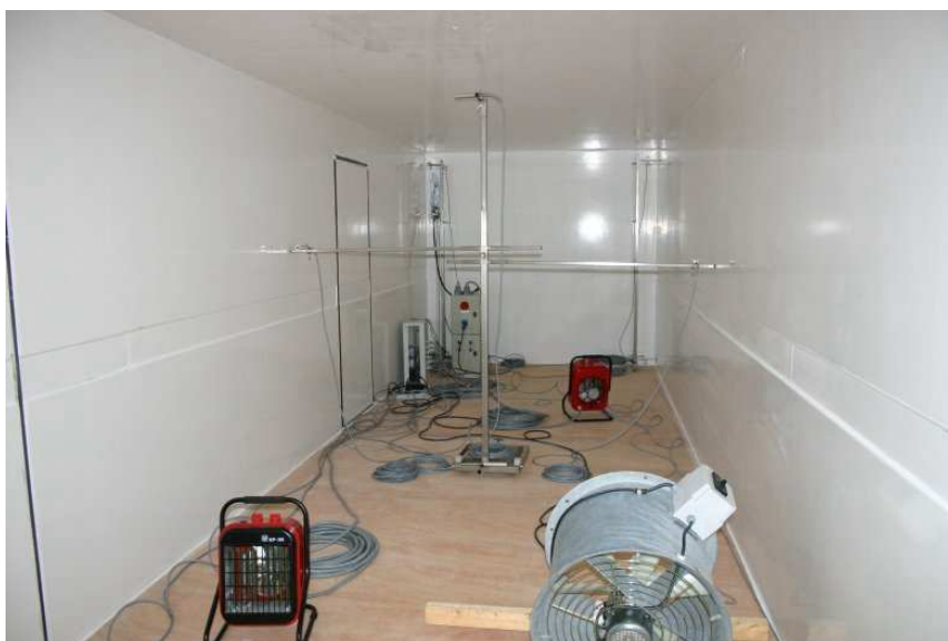
Fig. 4, K-value measurement equipment inside test body.
