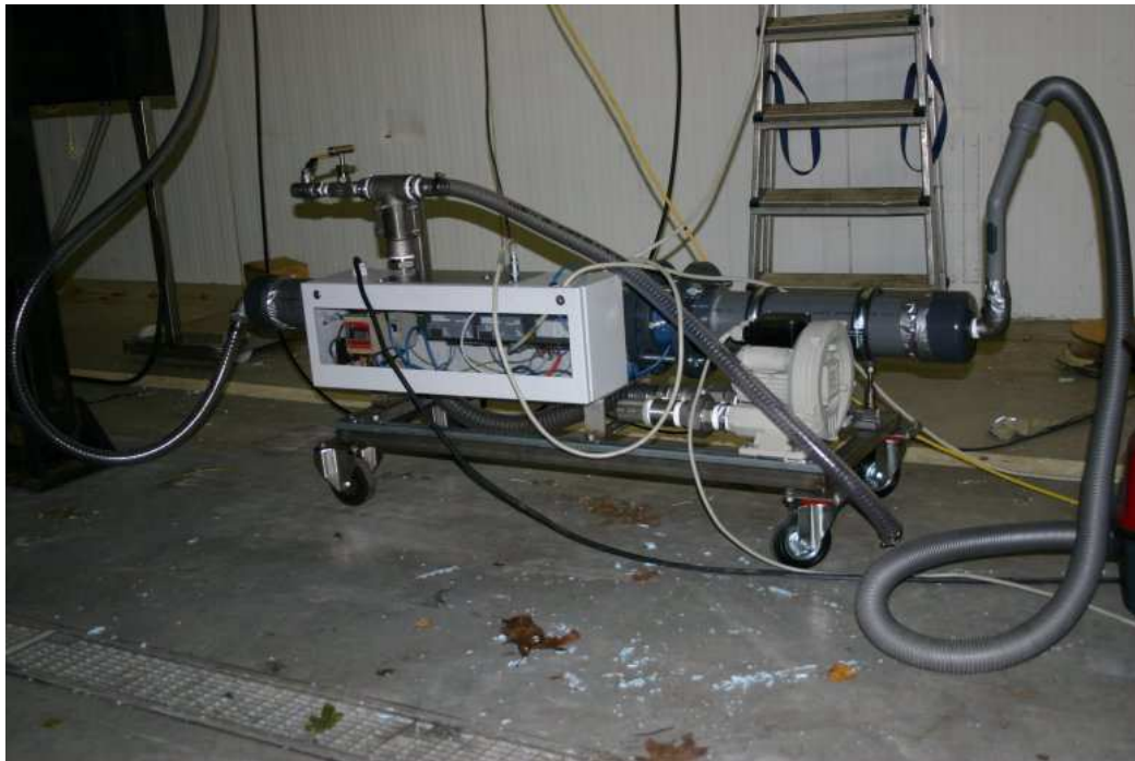
Fig. 5, air leakage measurement device.
