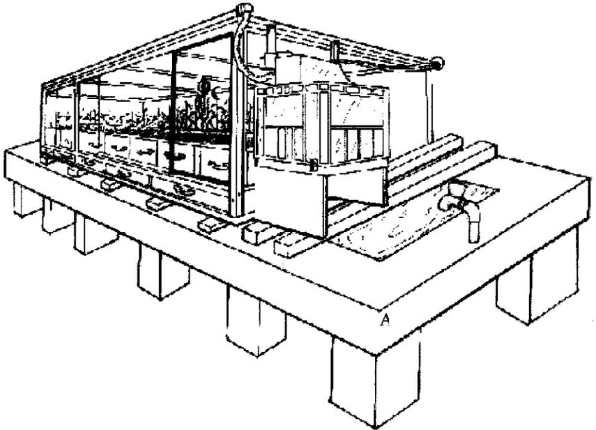
Figure 2-3 In "controlled" conditions the water was circulated through an automatic system to keep inside air temperature between 27° and 30° C. A = concrete table, B = small aquarium pump, C = thermostat.
