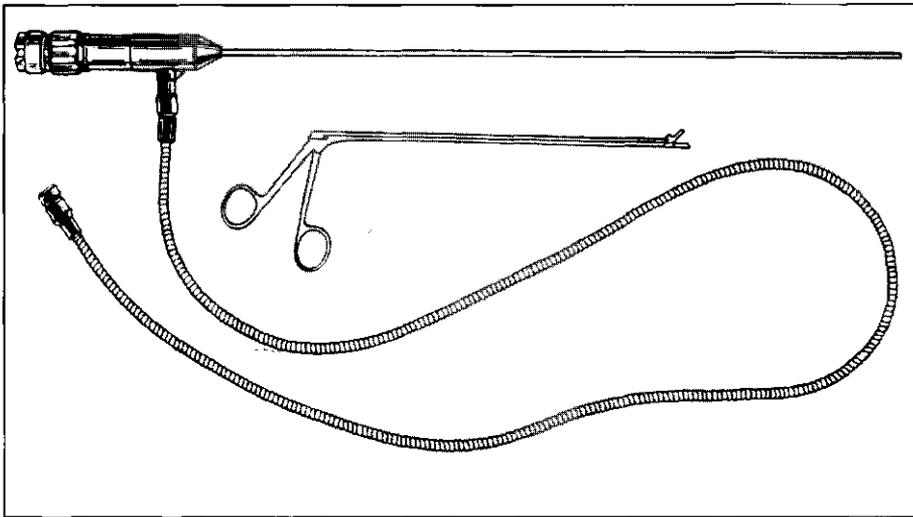
Figure 3-2 An intrascope (non-flexible endoscope) with flexible optical glass fibre connector to guide the light beam and medical biopsy forceps. The length of the thin tube that is to enter the perforations and the length of the biopsy forceps should fit the depth of the perforations (from Smits, 1994).
