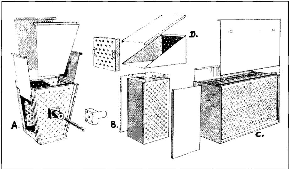
Figure 3-1 Four types of "perforons" suitable for use with the horizontally perforated soil system (from Smits, 1994)
