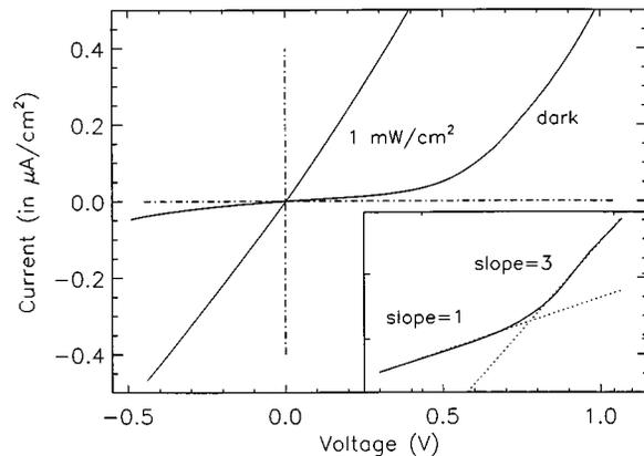
FIG. 7. I–V curves of a 100 nm single ZnTHOPP film in the dark and under  $1 \text{ mW/cm}^2$  AM1.5 illumination. In the inset the dark curve of  $\log(I)$  vs  $\log(V)$  shows the transition from linear to supralinear behavior.
