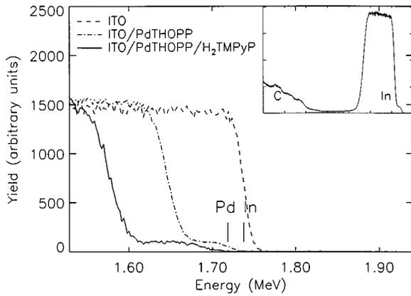
FIG. 2. RBS spectra of the indium edge of bare ITO and ITO substrates covered with a PdTHOPP single film and a H<sub>2</sub>TMPyP/PdTHOPP A/D heterojunction film. In the inset the total RBS spectrum of the single porphyrin film is shown (2.0 MeV He,  $\theta=170^\circ$  and  $\alpha=25^\circ$ ).
