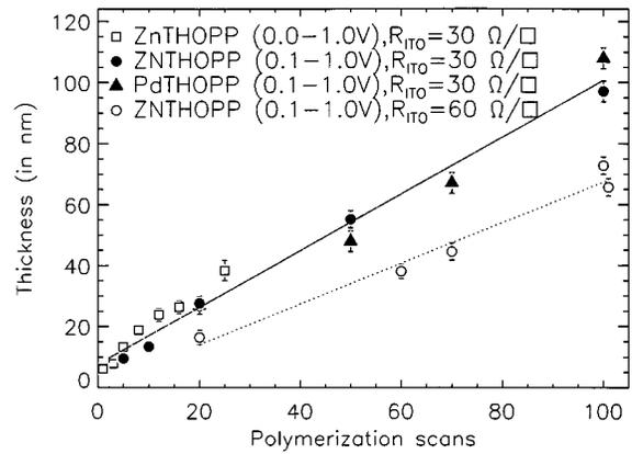
FIG. 4. Thickness of various polymer layers vs the number of polymerization scans.
