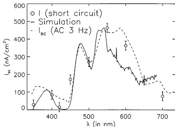
FIG. 13. Photoaction spectrum of a PdTHOPP/H<sub>2</sub>TMPyP heterostructure. The data are fitted to Eq. (16). A photoaction spectrum measured using a monochromator and a lock-in amplifier at 3 Hz is scaled to the spectrum measured with filters.
