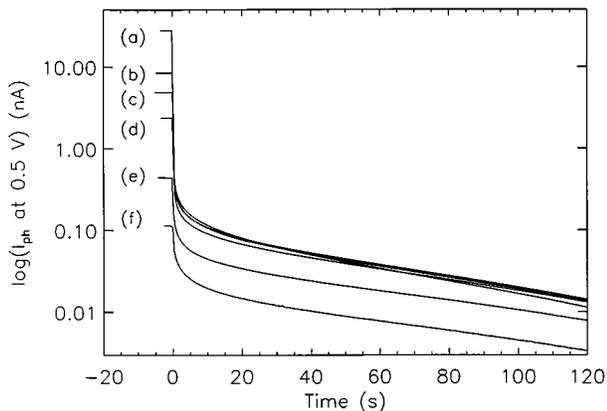
FIG. 9. Transient of the current at +0.5 V of a ~90 nm PdTHOPP single layer after switching off the light at various intensities. (a) 100 mW/cm<sup>2</sup>; (b) 21 mW/cm<sup>2</sup>; (c) 10 mW/cm<sup>2</sup>; (d) 3 mW/cm<sup>2</sup>; (e) 0.3 mW/cm<sup>2</sup>; (f) 0.1 mW/cm<sup>2</sup>.
