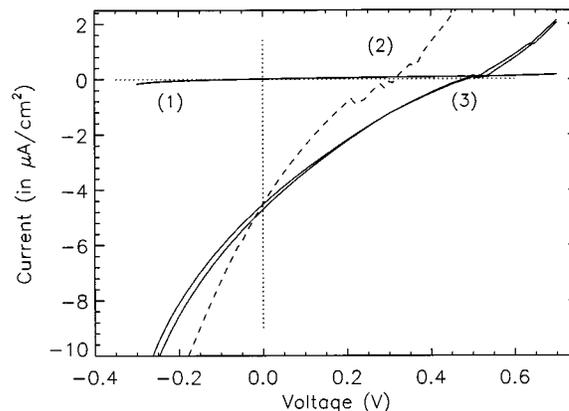
FIG. 11. I-V curves of a ITO/PdTHOPP(130 nm)/H<sub>2</sub>TMPyP(25 nm)/Ag heterojunction in dark and under 100 mW/cm<sup>2</sup> (AM1.5) illumination. Voltage scans (from -V to +V) are made at different speeds. (1) Dark curve; (2) voltage scan 0.01 V/s; (3) voltage scan 0.001 V/s.
