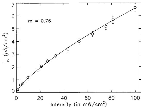
FIG. 12. Short-circuit current  $I_{sc}$  of an ITO/PdTHOPP(130 nm)/H<sub>2</sub>TMPyP(25 nm)/Ag heterojunction vs illumination intensity.
