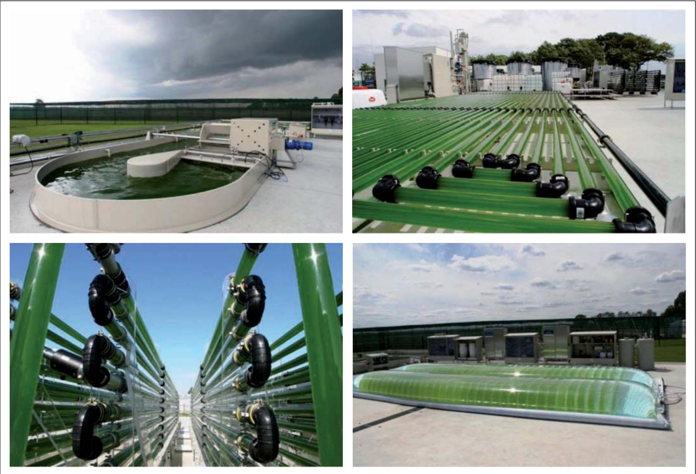
The four types of reactor systems at AlgaePARC (left to right, top to bottom): open raceway pond, horizontal tubular reactor, vertically stacked tubular reactor and flat panel reactor. Photos: AlgaePARC
