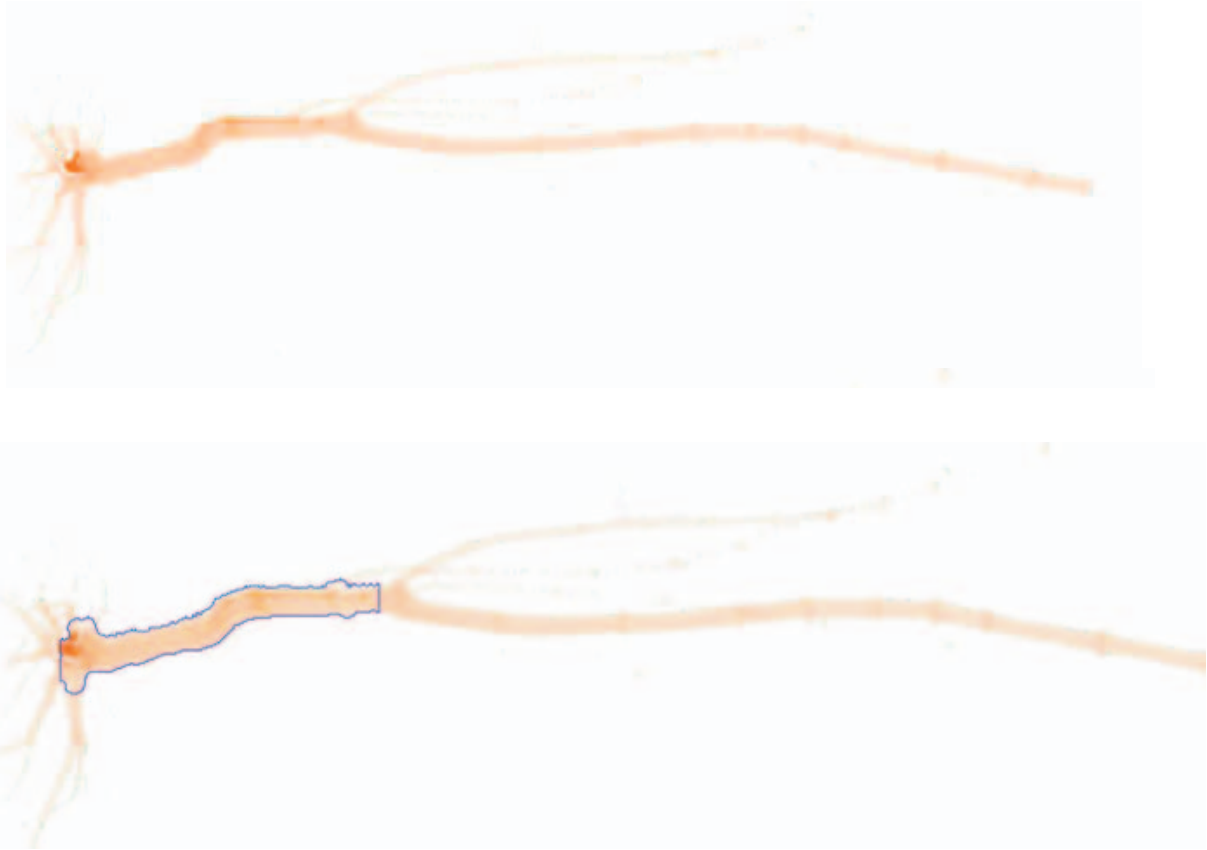
Figure 8. Example of a false negative in the validation dataset. Top original X-ray image; Bottom borehole detection after validation of the borehole detection method.
