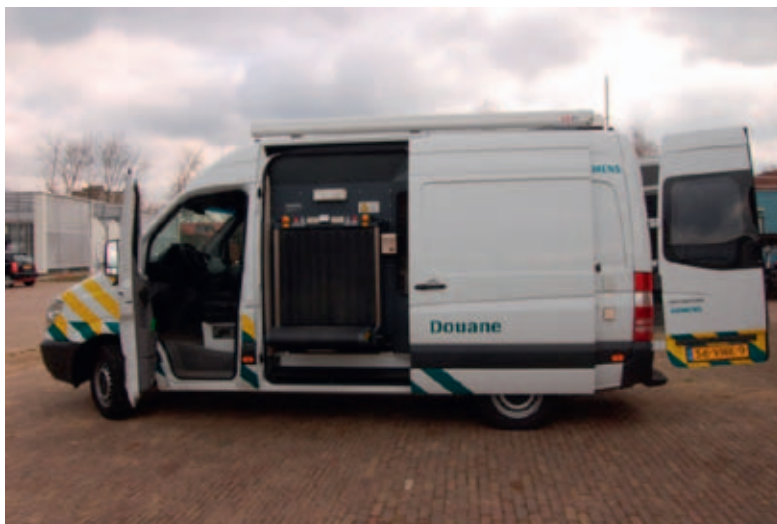
Figure 11. Transportable X-ray instrument currently in use by the Dutch Customs Laboratory.
