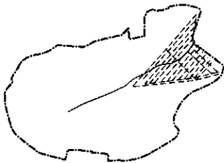
Fig. 5.12. The old ingrown drains of Raheenmore Bog (dashed lines) with position of the flow line to the margin in the ENE.
