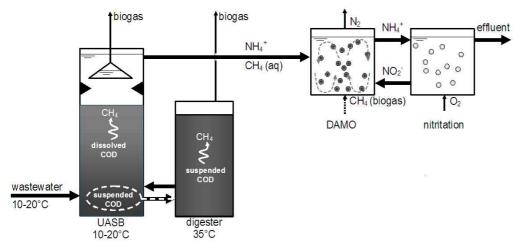
**Figure 1.** Proposed system configuration for anaerobic sewage treatment at low temperatures, consisting of a UASBdigester system, a reactor for nitrogen and methane removal by means of denitrification coupled to anaerobic methane oxidation (abbreviated as DAMO) and nitritation; adapted from Hendrickx *et al.* (2010).
