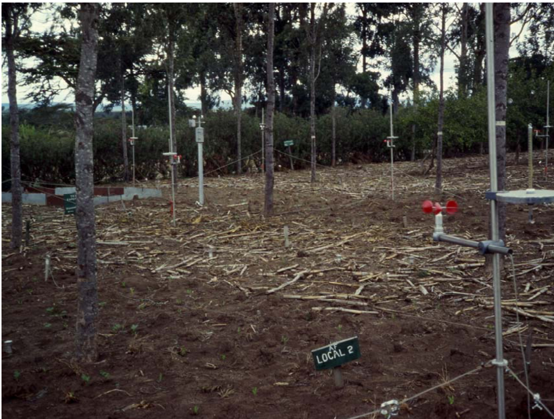
Figure 7. Cup anemometers and shaded Piche evaporimeters as ancillary anemometers in farmer demonstration projects in Matanya, Central Kenya. [Photo Kees Stigter]
