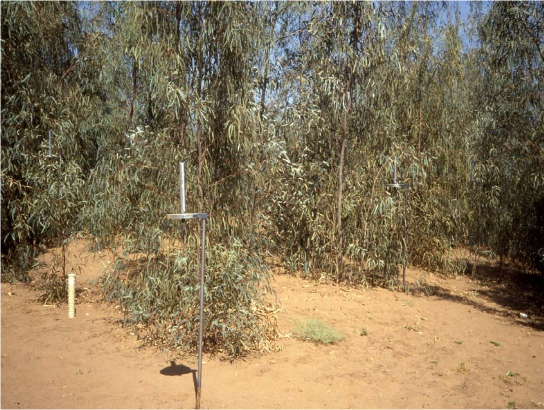
Figure 2B. Close up of the shelterbelt of Figure 2A, with equipment for measuring saltating sand and integrated wind speed with a shaded Piche evaporimeter. [Photo Kees Stigter]
