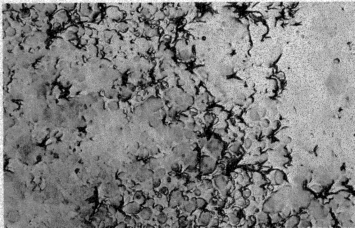
Fig. 93. Cuticular surface structure after a 5 min stay in water of 70° C. Replica technique used. (20,000 ×, t.e.m.)
