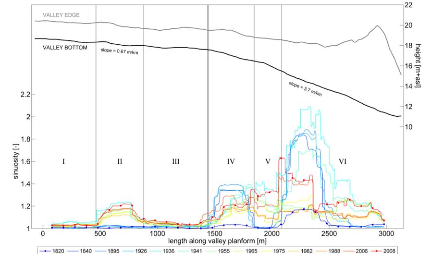
Figure 4. Along valley characteristics. Valley edge (gray line) and valley bottom (black line) are obtained from DEM analysis and correspond with the gray and black lines in Figure 2. Sinuosity (colored lines) are calculated according to Figure 5.
