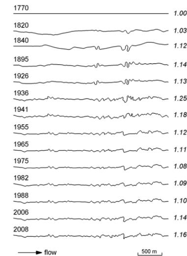
Figure 3. Historical channel planform change since 1820, shown in curvilinear coordinates. Sinuosity values shown in italics.
