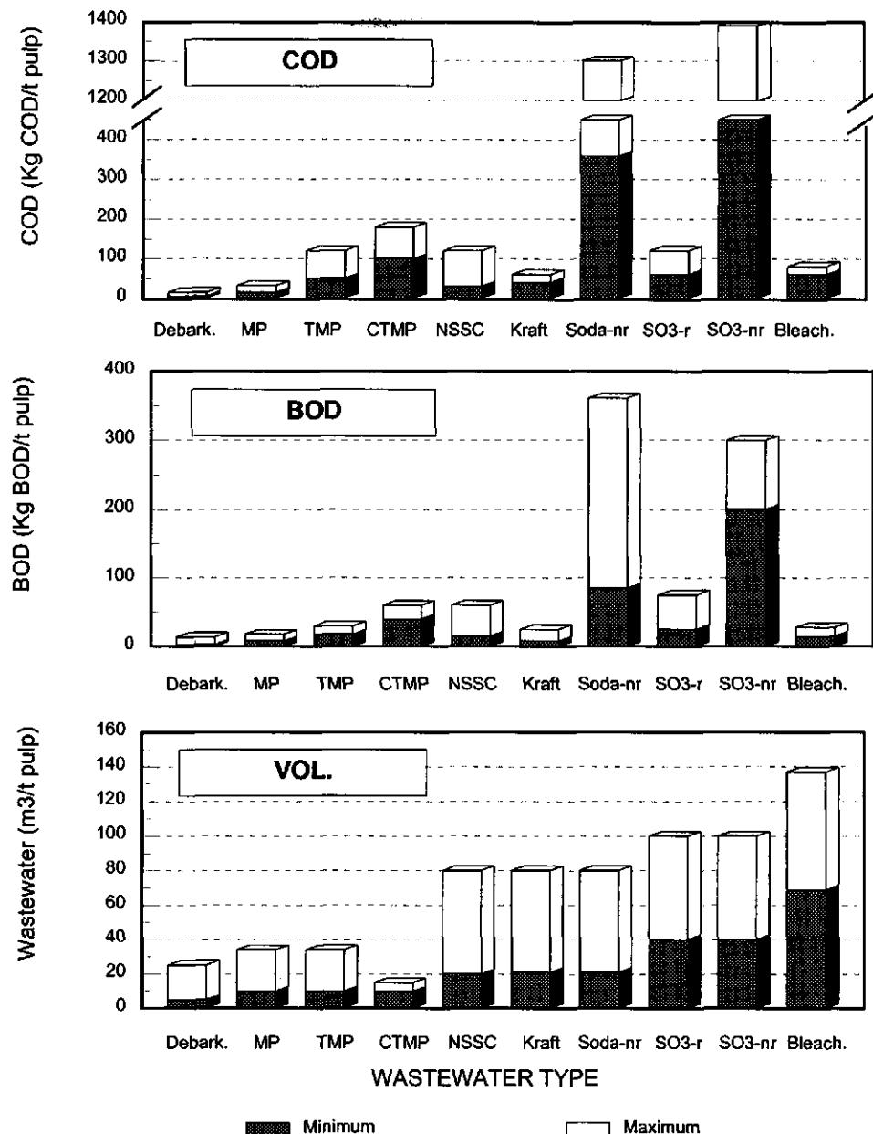
**Figure 3.** The specific pollution load of various wood-based pulping processes.
