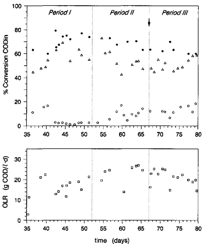
**Figure 3.** Performance of UASB reactor fed with hemp bark TMP wastewater. •) COD removal, % COD<sub>in</sub>; △) methanogenesis, % COD<sub>in</sub>; ○) VFA in effluent, % COD<sub>in</sub>; □) OLR, g COD·l<sup>-1</sup>·d<sup>-1</sup>. Arrow indicates partial removal of sludge from the UASB reactor (see Table 3).
