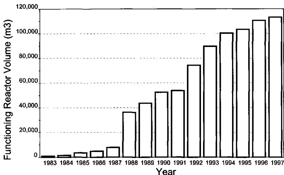
Figure 4. Functioning volume of anaerobic reactors in pulp and paper industry.
