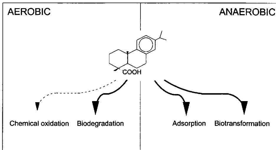
Figure 7. Fate of resin acids in aerobic and anaerobic treatment plants.
