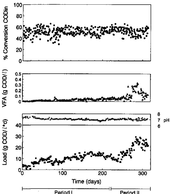
**Figure 2.** Operation and efficiency during anaerobic treatment of hemp bark black liquor. •) COD removal, % COD<sub>in</sub>; ○) methanogenesis, % COD<sub>in</sub>; ▲) VFA in effluent, % COD<sub>in</sub>; \*) pH in UASB reactor; ■) OLR, g COD·t<sup>-1</sup>d<sup>-1</sup>. Period I: day 0-220, COD<sub>in</sub> ≈ 1.9 g COD/l; Period II: day 221-316, COD<sub>in</sub> ≈ 3.9 g COD/l.
