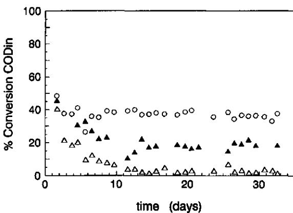
**Figure 3.** Performance of UASB reactor during anaerobic treatment of 12 g COD/l hemp stem wood black liquor without upfront dilution (experiment I). △) Methanogenesis, % COD<sub>in</sub>; ○) Acidification, % COD<sub>in</sub>; ▲) COD removal, % COD<sub>in</sub>; average OLR: 13.4 g COD/l-d.
