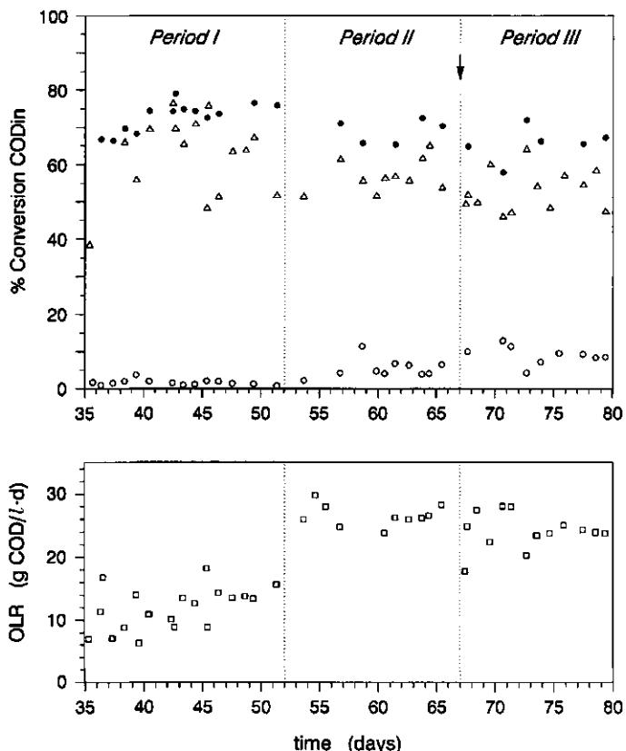
**Figure 2.** Performance of UASB reactor fed with hemp stem wood TMP wastewater. •) COD removal, % COD<sub>in</sub>; △) methanogenesis, % COD<sub>in</sub>; ○) VFA in effluent, % COD<sub>in</sub>; □) OLR, g COD· $t^{-1}d^{-1}$ . Arrow indicates partial removal of sludge from the UASB reactor (see Table 3).
