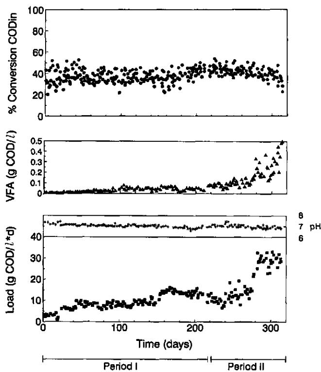
**Figure 3.** Operation and efficiency during anaerobic treatment of hemp stem wood black liquor. •) COD removal, % COD<sub>in</sub>; ○) methanogenesis, % COD<sub>in</sub>; ▲) VFA in effluent, % COD<sub>in</sub>; \*) pH in UASB reactor; ■) OLR, g COD·l<sup>-1</sup>d<sup>-1</sup>. Period I: day 0-220, COD<sub>in</sub> ≈ 1.9 g COD/l; Period II: day 221-316, COD<sub>in</sub> ≈ 3.9 g COD/l.
