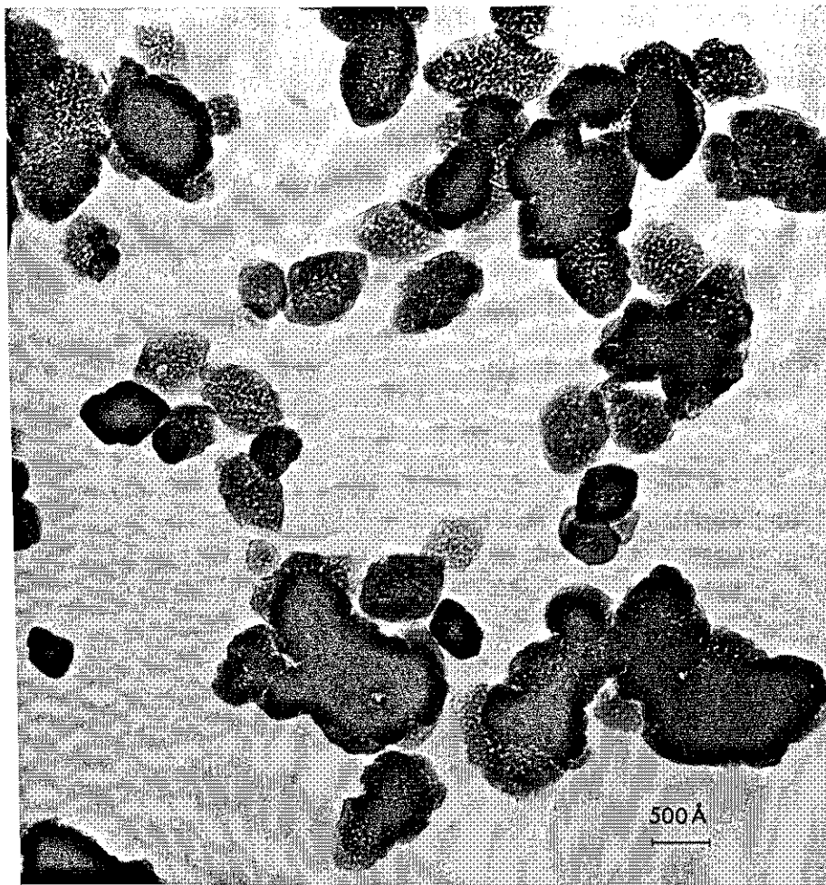
FIG. 2-3 Electron micrograph of hematite, sample A_d . Total magnification: 128,000 \times . By courtesy of Unilever Research Laboratory, Vlaardingen.
