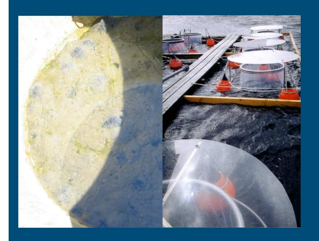
Flow-through marine mesocosms for testing contaminated sediment
